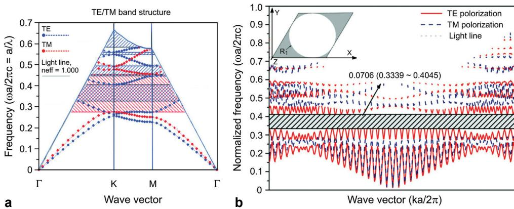
Fig. 2. The optimized structure with one circular hole in its unit cell and the corresponding band diagram for TM mode (solid lines) and TE mode (dotted lines);  $\Gamma$ ,  $K$ , and  $M$  refer to the corner points of the 1/8 Brillouin zone – **a**. The optimized structure with one circular hole in its unit cell and the corresponding band diagram for TE and TM polarizations of full zone – **b**.
