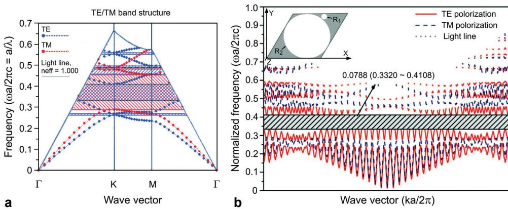
Fig. 3. The optimized structure with two circular holes in its unit cell and the corresponding band diagram for TM mode (solid lines) and TE mode (dotted lines);  $\Gamma$ ,  $K$ , and  $M$  refer to the corner points of the 1/8 Brillouin zone – a. The optimized structure with two circular holes in its unit cell and the corresponding band diagram for TE and TM polarizations of full zone – b.
