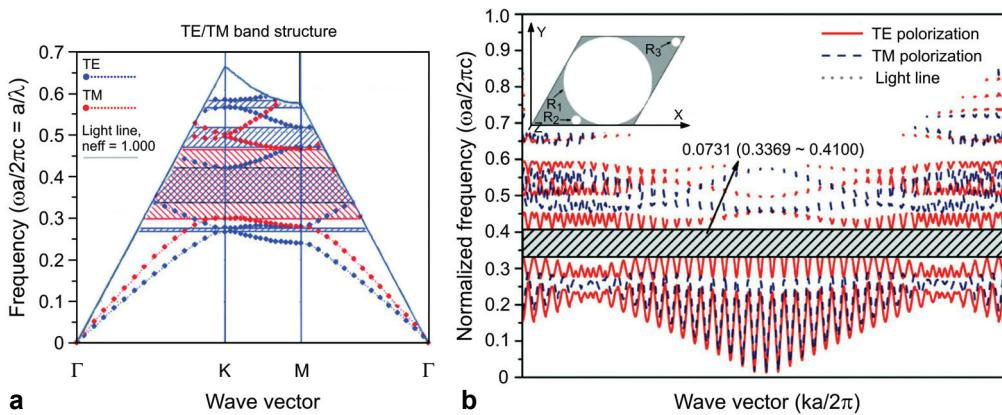
Fig. 4. The optimized structure with three circular holes in its unit cell and the corresponding band diagram for TM mode (solid lines) and TE mode (dotted lines);  $\Gamma$ ,  $K$ , and  $M$  refer to the corner points of the 1/8 Brillouin zone – a. The optimized structure with three circular holes in its unit cell and the corresponding band diagram for TE and TM polarizations of full zone – b.
