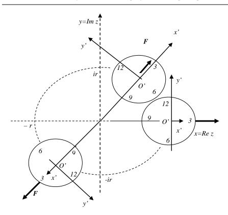
Fig. 4. Fictitious force - the centrifugal force
