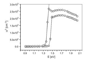
Fig. 1. The square of the absorption coefficient  $\alpha^2$  as a function of photon energy hv for CdTe:Ga at room temperature (open circles) and at 77 K (open squares). The solid lines are the best square linear fits to the experimental data.
