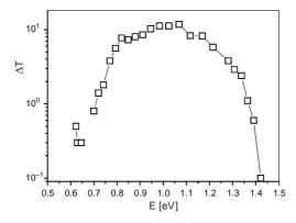
Fig. 5. The difference  $\Delta T$  between the transmission spectra measured in darkness and after illumination at 77 K, related to the data shown in Fig. 4.
