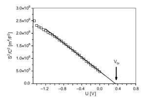
Fig. 2. Capacitance–voltage characteristic for CdTe:Ga measured at 300 K. The solid line is the best square linear fit to the experimental data. The fit yields the value of built in voltage equal to 0.33 eV and donor net concentration equal to  $10^{17}$  cm<sup>-3</sup>.
