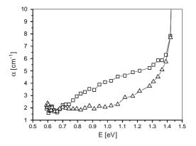
Fig. 4. Optical absorption for CdTe:Ga at 77 K (open triangles) and after preliminary 30 min illumination with halogen light (open squares). The latter measurements were performed 10 min after termination of light.
