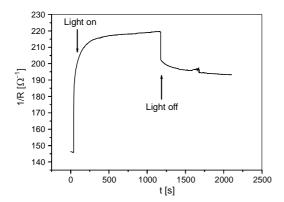
Fig. 3. Conductivity build-up and decay for CdTe:Ga at 77 K. The sample was illuminated with photons of energy equal to 1.24 eV.
