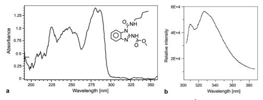
Fig. 8. Absorption spectrum (**a**) and fluorescence spectrum (**b**) of  $1 \times 10^{-3}$  M benomyl in CH<sub>3</sub>CN, ( $\lambda_{exc} = 290$  nm).
