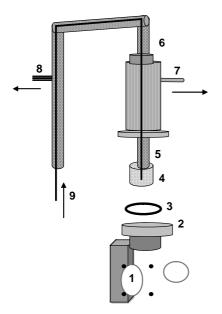
Fig. 2. Open cycle liquid nitrogen cryostat: 1 – aluminum block with quartz windows, 2 – Varian type adapter, 3 – Rubber O-ring, 4 – metal block with drilled volume to receive liquid nitrogen and to act as a heat exchanger, 5 – liquid nitrogen transfer line, 6, 7 – stainless steel cylinder with vacuum outlet, 8 – vacuum outlet to evacuate the transfer line, 9 – capillary tube for liquid nitrogen inlet.
