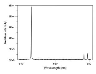
Fig. 5. Mercury spectral lines acquired using the high resolution grating (300 grooves/mm).
