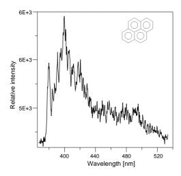
Fig. 6. Fluorescence spectrum of  $1.0 \times 10^{-6}$  g/l pyrene in cyclohexane at room temperature obtained with a single 15 nsec duration laser pulse at 337.1 nm using N<sub>2</sub> laser excitation source.
