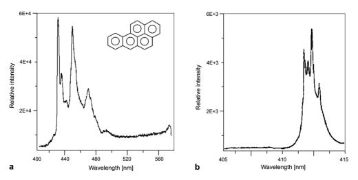
Fig. 7. Room temperature low resolution fluorescence spectrum (**a**) and low temperature ( $-150^{\circ}$ C) high resolution fluorescence spectrum (**b**) of  $2.0 \times 10^{-5}$  g/l benzo(a)pyrene in n-heptane ( $\lambda_{exc} = 337$  nm).
