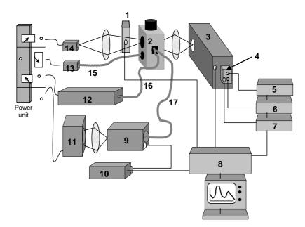
Fig 1. Block diagram of the experimental set-up: 1 - electromechanical shutter, 2 - sample cell holder, 3 - spectrograph, 4 - CCD unit, 5 - fast high voltage pulser, 6 - detector controller, 7 - delay generator, 8 - computer, 9 - excitation monochromator, 10 - excitation monochromator drive unit, 11 - xenon lamp, 12 - nitrogen laser, 13 - tungsten lamp, 14 - deuterium lamp, and 15, 16, 17 - 1 mm UV passive optical fiber.
