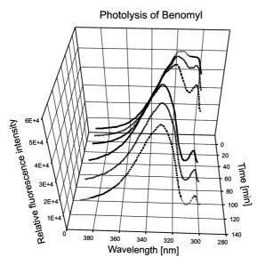
Fig. 9. Fluorescence spectrum of benomyl CH<sub>3</sub>CN solution at different times of photolysis ( $\lambda_{exc} = 290 \text{ nm}$ ).
