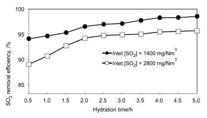
Fig. 5. Effect of hydration time on the SO<sub>2</sub> removal efficiency
