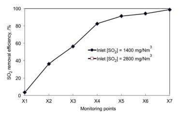
Fig. 6. SO<sub>2</sub> removal efficiency along the vertical direction of the reactor
