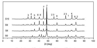
Fig. 2. X-ray diffraction pattern of the modified sorbents: 1 – NaOH, 2 – SiO<sub>2</sub>, 3 – Ca<sub>4</sub>Al<sub>8</sub>Si<sub>8</sub>O<sub>32</sub>, 4 – Ca<sub>1.5</sub>SiO<sub>3.5</sub>, 5 – Na<sub>2</sub>Si<sub>2</sub>O<sub>5</sub>, 6 – CaSiO<sub>3</sub>, 7 – Ca(OH)<sub>2</sub>, Fe<sub>2</sub>O<sub>3</sub>
