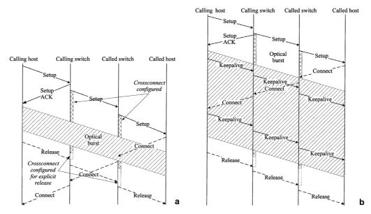
Fig. 1. Supported connection types: short burst (a), lightpath (b).
