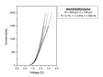
Fig. 5. Current-voltage characteristic of the semiconductor laser grown in the optimum growth conditions.
