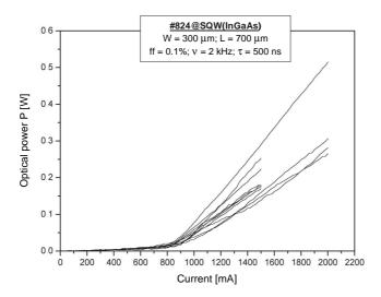
Fig. 6. Light-current characteristic of the semiconductor laser grown in the optimum growth conditions.
