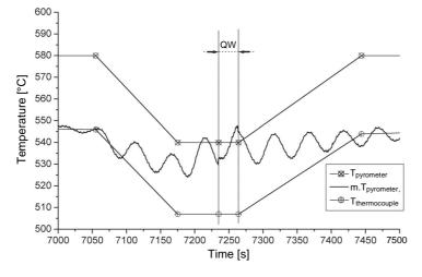
Fig. 2. Substrate temperatures during the growth process of the active region of the semiconductor laser for a 980 nm band. (+) and  $(\times)$  are assumed temperatures measured by a thermocouple and by a pyrometer, respectively. Solid line without marks is the real temperature registered by a pyrometer. The process has not been optimised.
