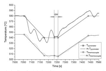
Fig. 3. Effect of optimisation of the growth process of the semiconductor laser for a 980 nm band – the real temperature in the QW is almost constant. (+) and ( $\times$ ) are assumed temperatures measured by a thermocouple and by a pyrometer, respectively. Solid line without marks is the real temperature registered by a pyrometer, while the dashed one represents the temperature measured by a thermocouple.
