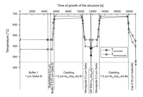
Fig. 1. Scheme of the structure of the semiconductor laser for a 980 nm band and the assumed growth temperatures measured by a thermocouple (+) and by a pyrometer  $(\times)$ .
