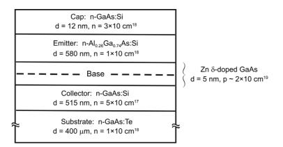
Fig. 1. Scheme of the layer structure used for HPT.
