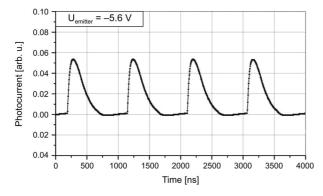
Fig. 6. Time response of the HPT for near breakdown bias voltage (-5.6 V).
