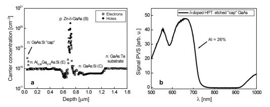
Fig. 2. EC-V profile of the HPT structure (a). PVS spectrum of the AlGaAs emitter layer (b).
