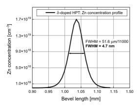
Fig. 3. Zinc distribution inside the base region estimated by micro-Raman spectroscopy.
