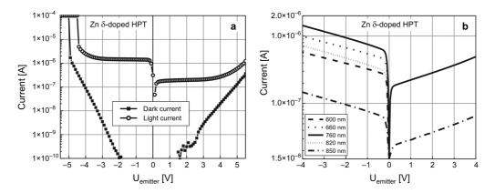
Fig. 5. Measured I-U characteristics of HPT (a). Simulated I-U characteristics of HPT structure (b).
