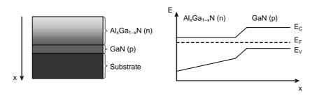
Fig. 4. Schematic structure of *p*-*n* photodiode with graded layer.
