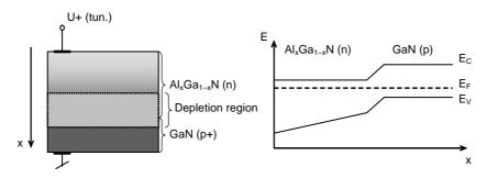
Fig. 5. Schematic structure of tunable photodetector.
