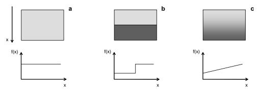
Fig. 1. Schematic representation of materials function in different structures; homogenous material (**a**), junction (**b**), FGM (**c**).
