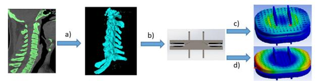
Fig. 1. The process of designing personalized product: a) obtain the geometry of vertebrae,b) modeling the implant geometry, c) maximum strength in the FEM simulation,d) maximum deformations in the FEM simulation
