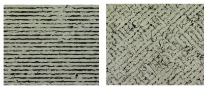
Fig. 1. Examples of crystalline (dark) – amorphous (white) composites obtained in the process
