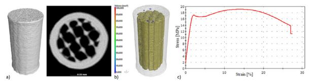
Fig. 1a), b) The result of CT reconstruction – 2D and 3D view, c) Stress-strain curve
