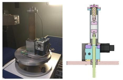
Fig. 1. Test device concept: adjustment in the CT (left) and scheme (right).
