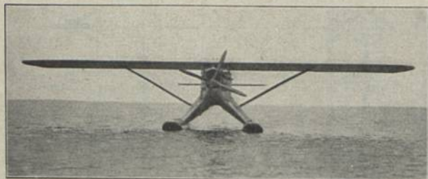
Kawasaki-Dornier Do D (1925) Kwj 2; E: C. Dornier b = 19,60 m; l = 12,72 m; T = 62,00 m 2 ; L = 2,00 t; N = 1,05 t; G = 3,05 t; V = 181 km/h; St = 3,0 km/32'; M: Napier 450 PS-HP-CV; Bst.: D, S.
