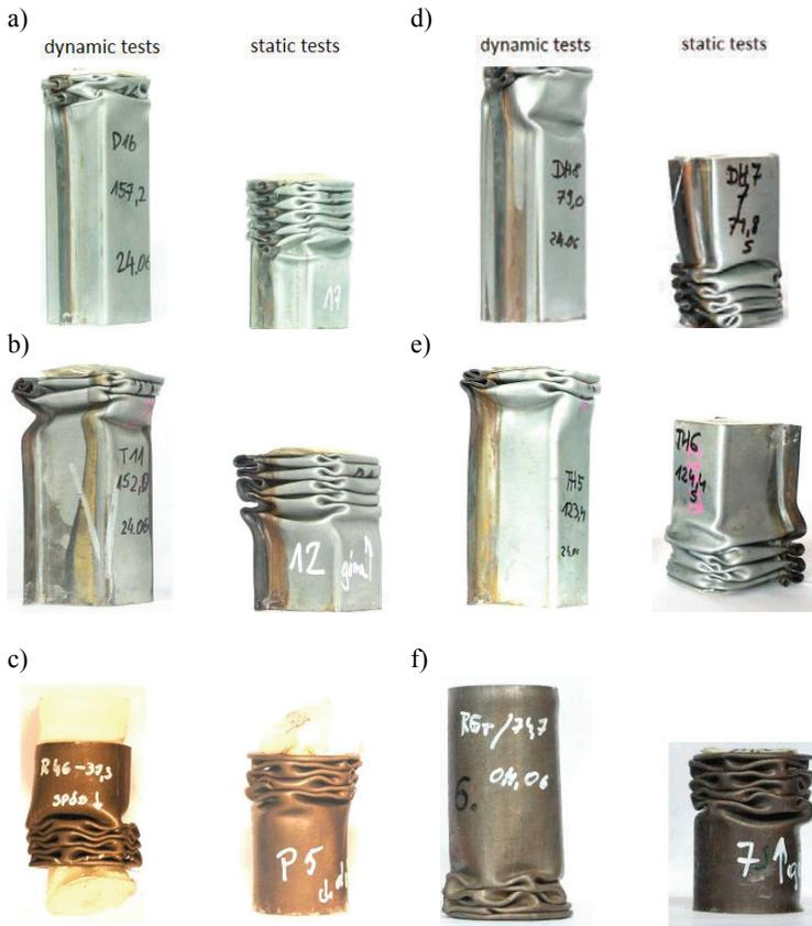
Fig. 11. Comparison of dynamic and static method of upsetting specimens: a) symmetric specimens with single wall and similar packing densities, b) asymmetric specimens with single wall and similar packing densities, c) tubular specimens with similar packing densities, d) asymmetric specimens with double wall and similar packing densities, f) specimens with double wall and similar packing densities [9]
