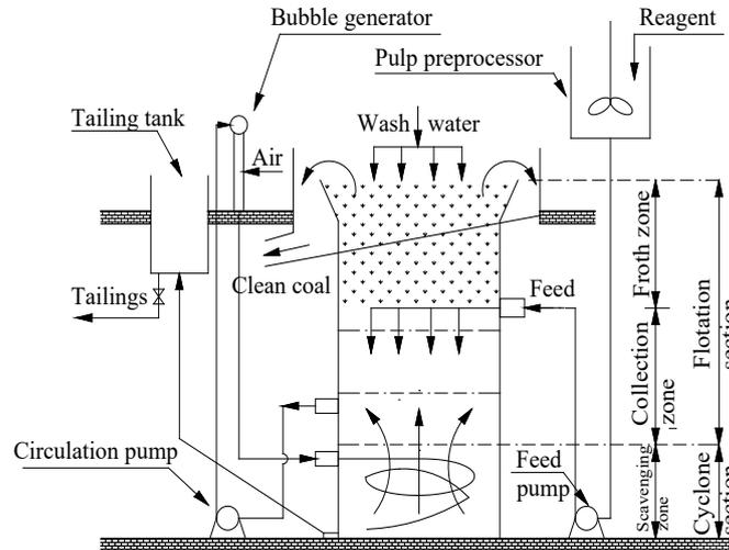
Fig. 1. Schematic illustration of the FCMC flotation column
