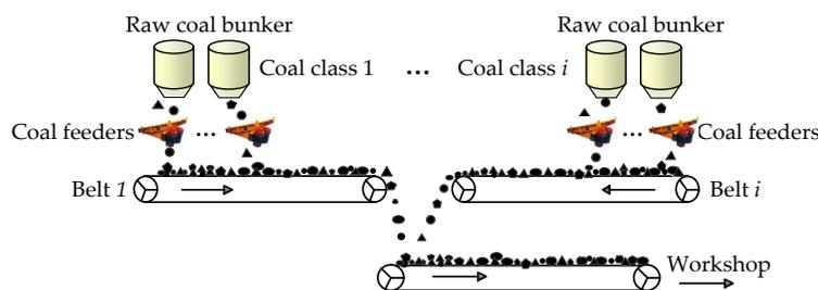
Fig. 2. Schematic illustration of coal blending process
