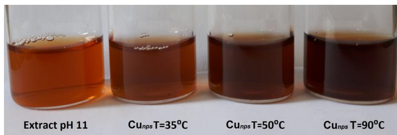
Fig. 3. Colour change of synthesized  $\text{Cu}_{\text{nps}}$  with a temperature of the reaction
