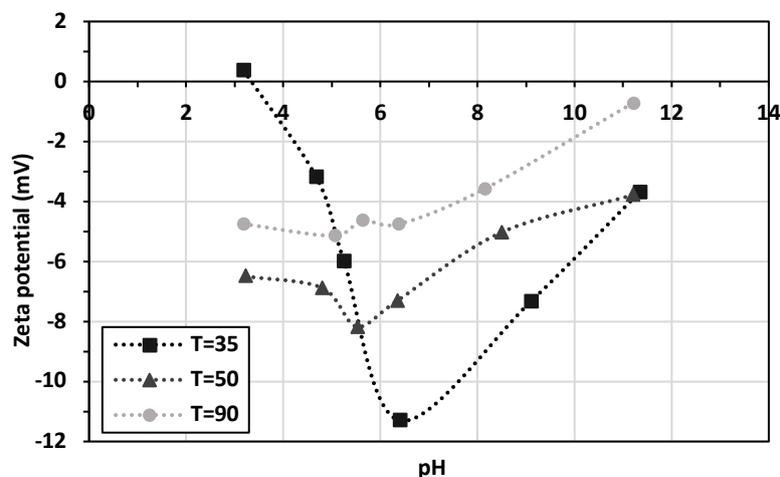
Fig. 6. Influence of the reaction temperature on the zeta potential of copper nanoparticles (aerobic conditions, Cu:E = 1:10, nanoparticles fabricated at pH 11)
