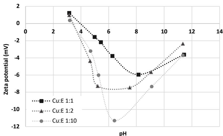
Fig. 1. Influence of reagent ratio on the zeta potential of copper nanoparticles ( $T=35^{\circ}\text{C}$ , pH 11)
