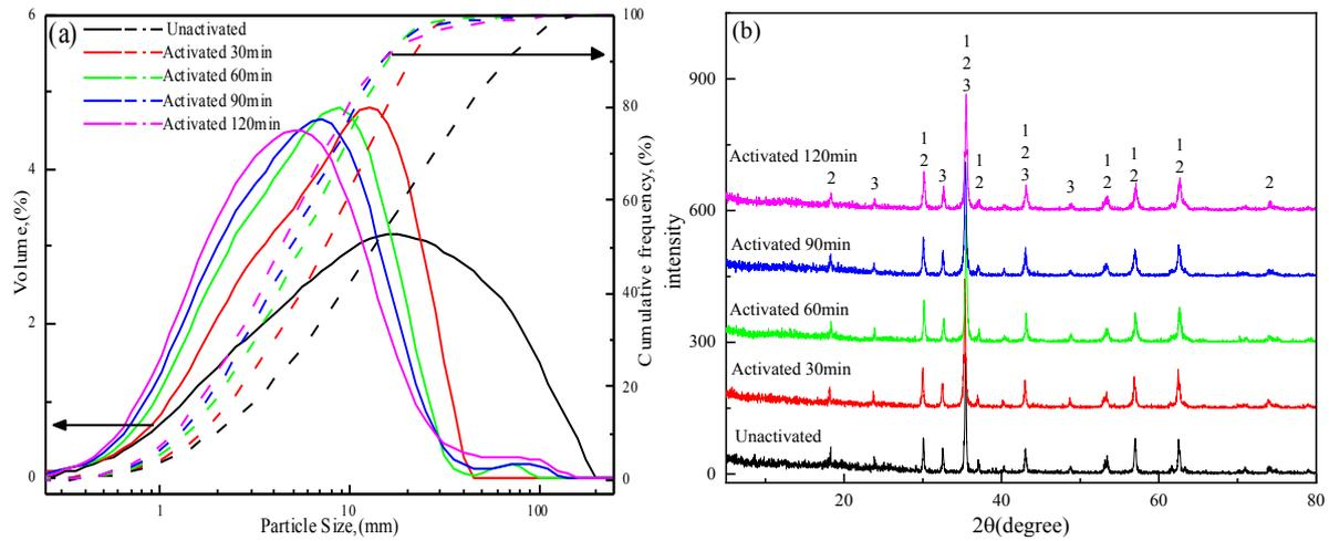
Fig. 1. (a) Particle size distribution as a function of activation time, (b) XRD patterns of the unactivated and activated samples (1- $\text{Fe}_{2.75}\text{Ti}_{0.25}\text{O}_4$ ; 2- $\text{Fe}_3\text{O}_4$ ; 3- $\text{FeTiO}_3$ )
