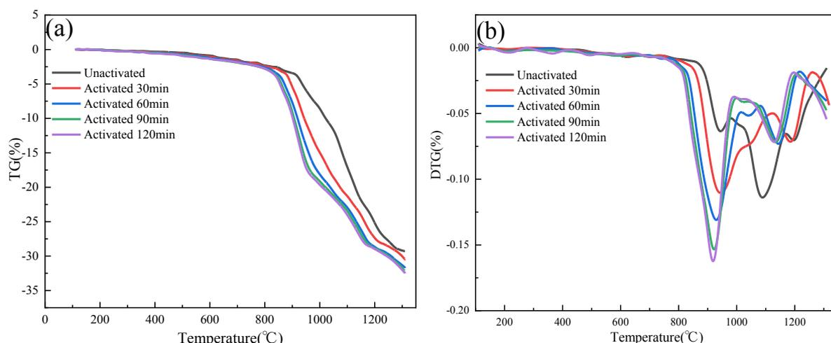
Fig. 4. Thermogravimetric results of samples with different activation times
