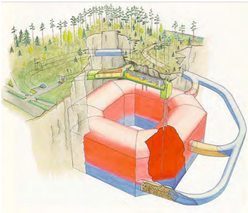
Fig. 2. Diagram of an underground thermal energy storage facility in Lyckebo, Sweden
