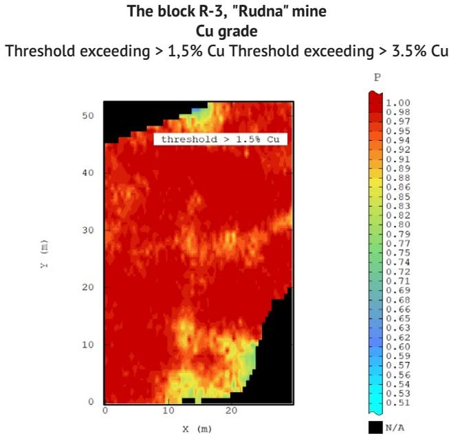
Fig. 34. Raster map of distribution of probability P values of threshold exceeding > 1.5 % Cu; Cu grade in the deposit, the R-3 block, "Rudna" mine
