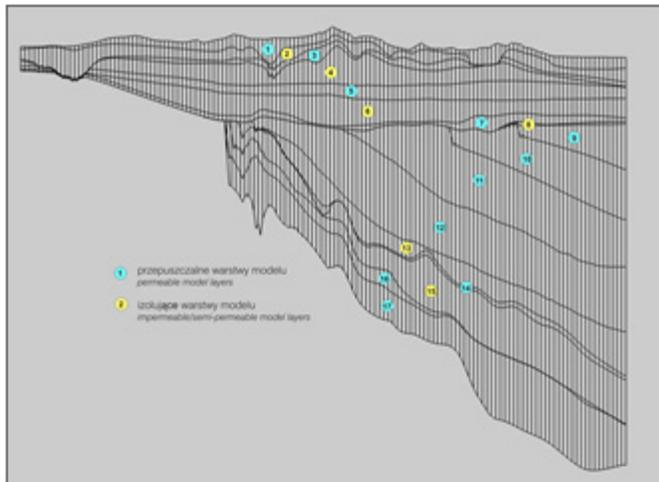
Fig. 2. Schematic system of aquifers and insulating layers separated on the numerical model of KGHM
