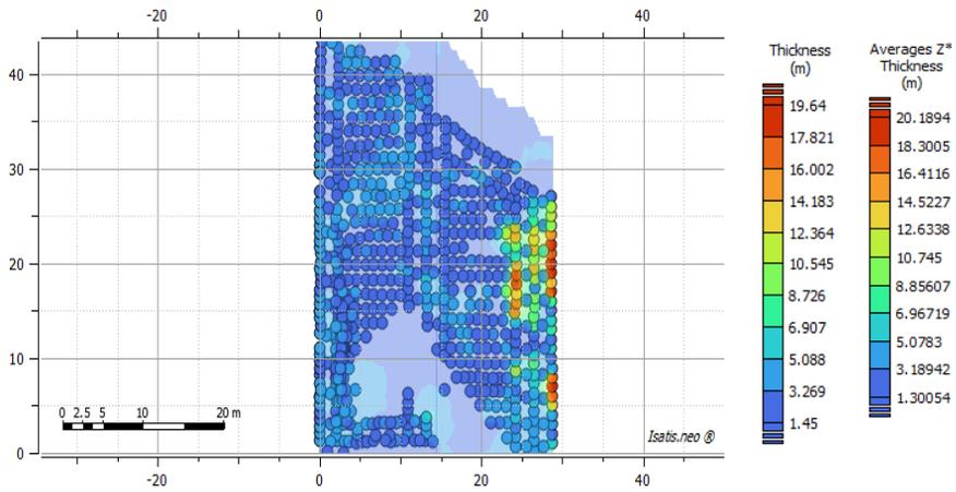
Fig. 18b. Raster map of distribution of estimated averages  $Z^*$  of thickness  $th$  [m] with sampling points (basemap); the block R-1, "Rudna" mine; the results of ordinary (block) kriging
