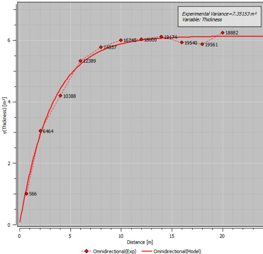
Fig. 13. Isotropic variogram of thickness  $[m]^2$ , approximated by theoretical functions in enclosed Cu ore deposit; with parameters of the assumed models: **cubic model**: range of influence  $a = 2.55$  m, sill variance  $C = 1.65$   $m^2$ ; **spherical model**: range of influence  $a = 9.57$  m, sill variance  $C = 4.37$   $m^2$ ; total sill variance  $C = 6.02$   $m^2$ ; the block R-1, "Rudna" mine
