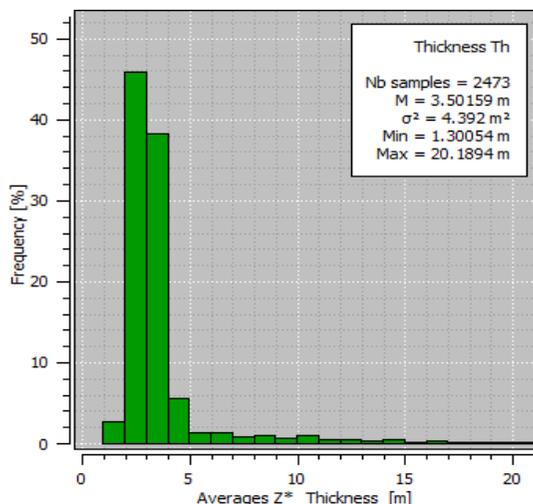
Fig. 20. Histogram of averages  $Z^*$  of thickness [m] distribution in enclosed Cu ore deposit; the block R-1, "Rudna" mine; skewness  $g_1 = 4.12$ , extremely strong asymmetry;  $g_2 = 22.87$ , a leptokurtic kurtosis; variation coefficient  $V = 59.85\%$
