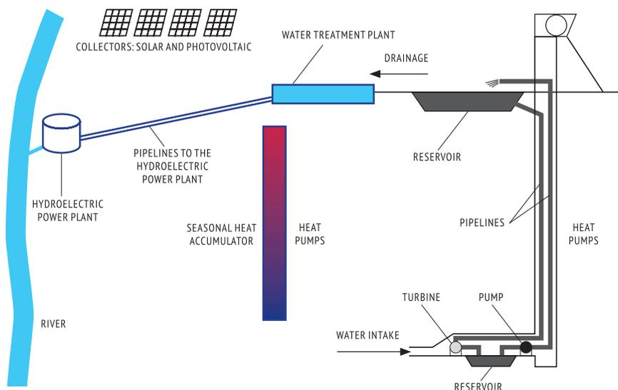
Fig. 1. Conversion of energy from renewable energy sources, using mine water (author's research)
