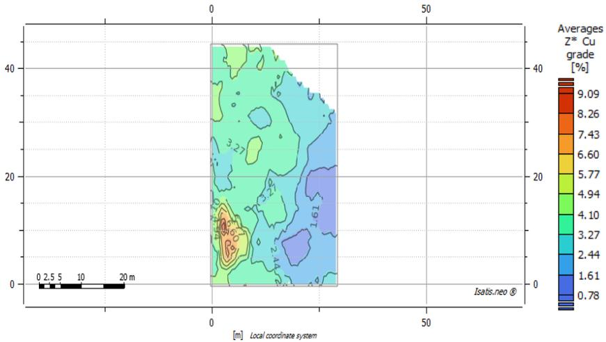
Fig. 17c. Isoline map of distribution of estimated averages  $Z^*$  of Cu grade [%]; the block R-1, "Rudna" mine; the results of ordinary (block) kriging
