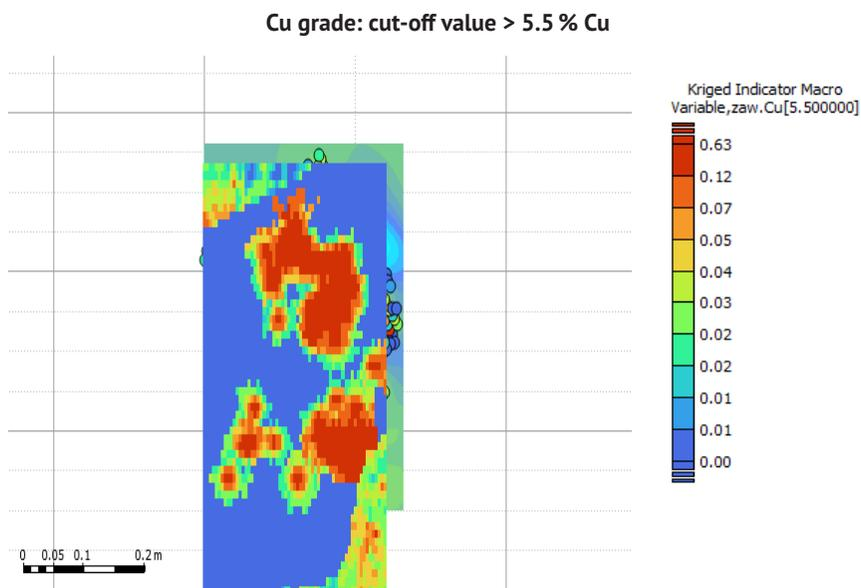
Fig. 33. Raster map of distribution of probability P of copper grade [%]: the cut-off value > 5.5 % Cu; the R-3 block; "Rudna" mine
