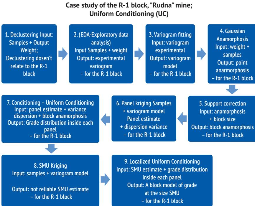
Fig 36. Uniform Conditioning (UC); Workflow; the R-1 block, "Rudna" mine.
