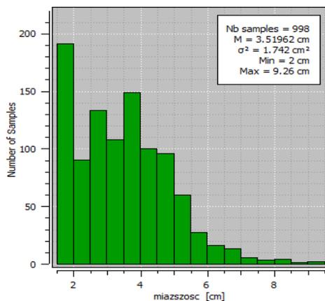
Fig. 27. Histogram of original values Z of thickness [m] distribution in enclosed Cu ore deposit; the block R-3, "Rudna" mine; skewness  $g_1 = 0.89$ , weak asymmetry;  $g_2 = 3.83$ , a leptokurtic kurtosis; variation coefficient  $V = 37.50\%$
