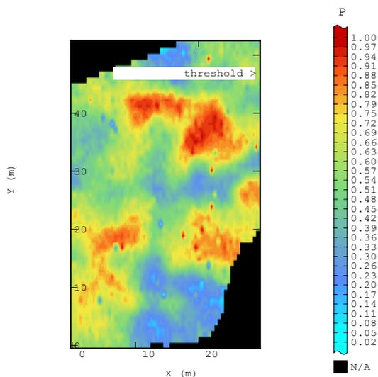
Fig. 35. Raster map of distribution of probability P values of threshold exceeding > 3.5 % Cu; Cu grade in the deposit, the R-3 block, "Rudna" mine.
