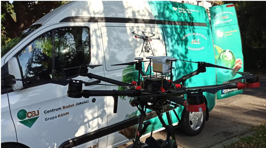
Fig. 7. An example of a measurement set – a drone armed with a portable air analyzer with a built-in air sampling module
