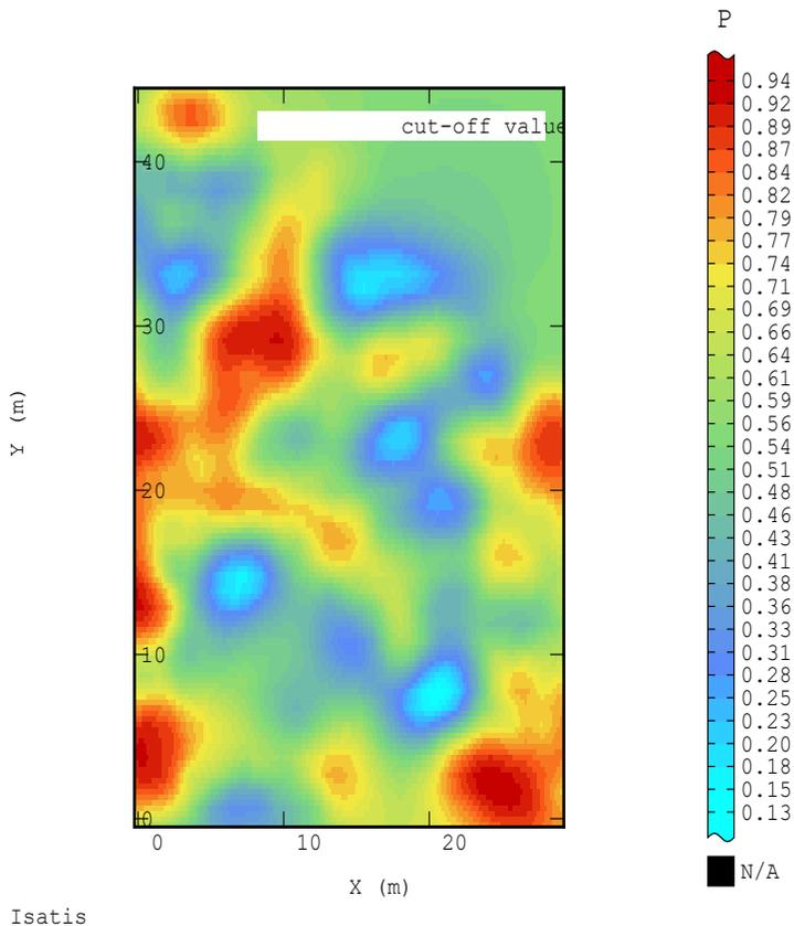
Fig. 22. Raster map of probability P distribution for the cut-off value > 2.5 m; thickness [m]; the R-1 block; "Rudna" mine
