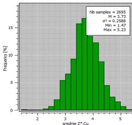
Fig. 30. Histogram of distribution of estimated averages Z\* of Cu grade [%]; the R-3 block, "Rudna" mine; skewness  $g_1 = 0.76$ , weak asymmetry;  $g_2 = 5.48$ , a leptokurtic kurtosis; variation coefficient  $V = 34.46\%$
