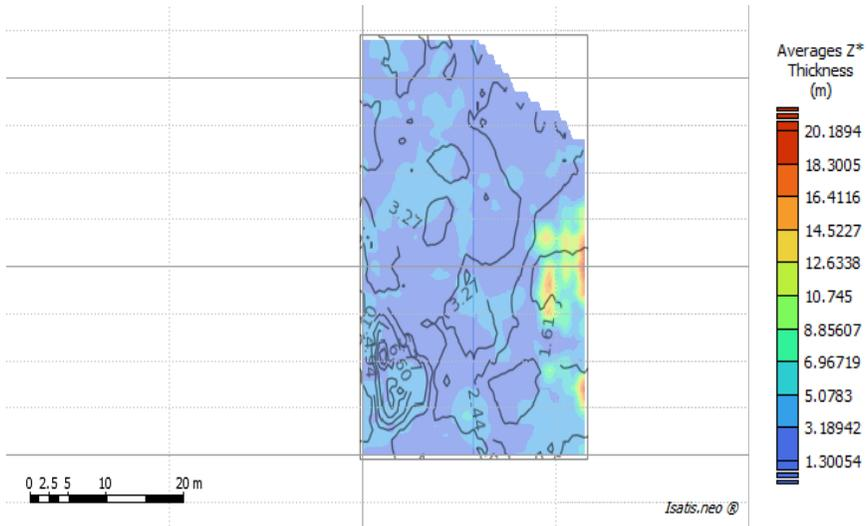
Fig. 18c. Isoline map of distribution of estimated averages  $Z^*$  of thickness  $th$  [m] with sampling points (basemap); the block R-1 "Rudna" mine; the results of ordinary (block) kriging
