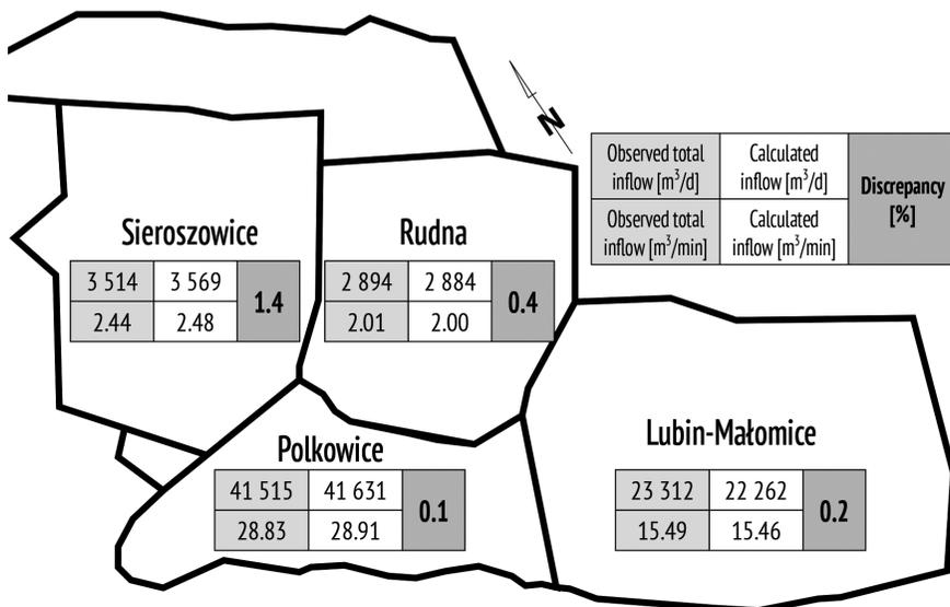
Fig. 3. Summary of the size of groundwater inflows to the workings observed and obtained on the model in m<sup>3</sup>/min
