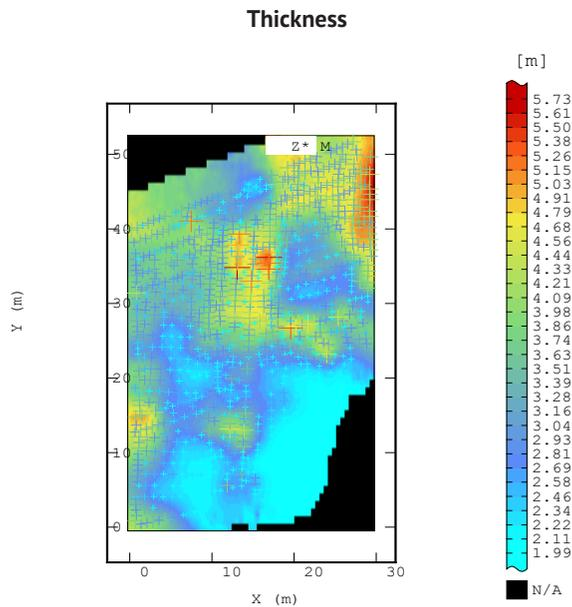
Fig. 29. Raster map of distribution of estimated averages  $Z^*$  of the thickness [m]; the R-3 block, "Rudna" mine
