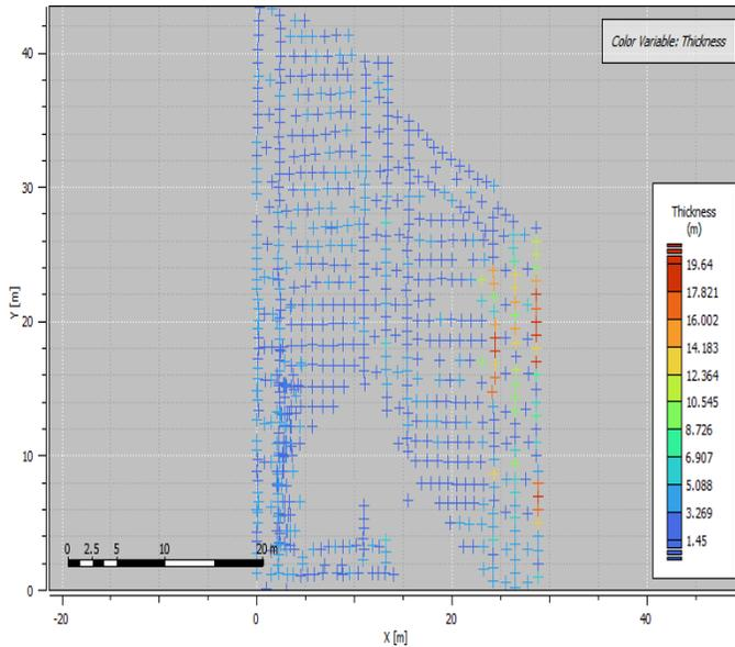
Fig. 6. Basemap with sampling points: thickness [m]; size N=708; distance between samples 15–20 m in the headings; The block R-1, "Rudna" mine
