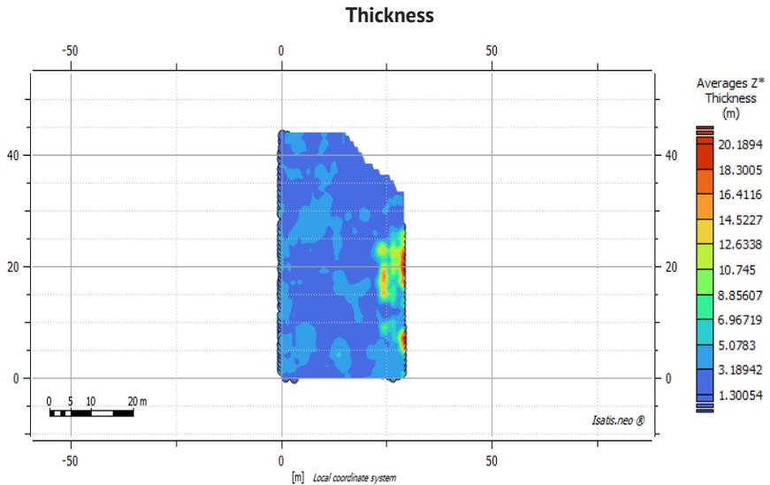
Fig. 18a. Raster map of distribution of estimated averages  $Z^*$  of thickness [m]; the block R-1, "Rudna" mine; the results of ordinary (block) kriging
