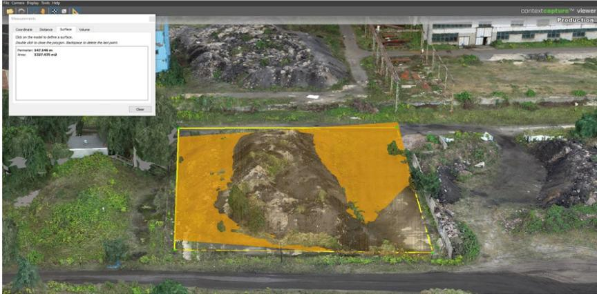
Fig. 6. An example of the use of drone raids equipped with a high-resolution camera. The analysis of photos specialized programs allows you to document the places of sampling or determine the size and location of potential sources of pollution
