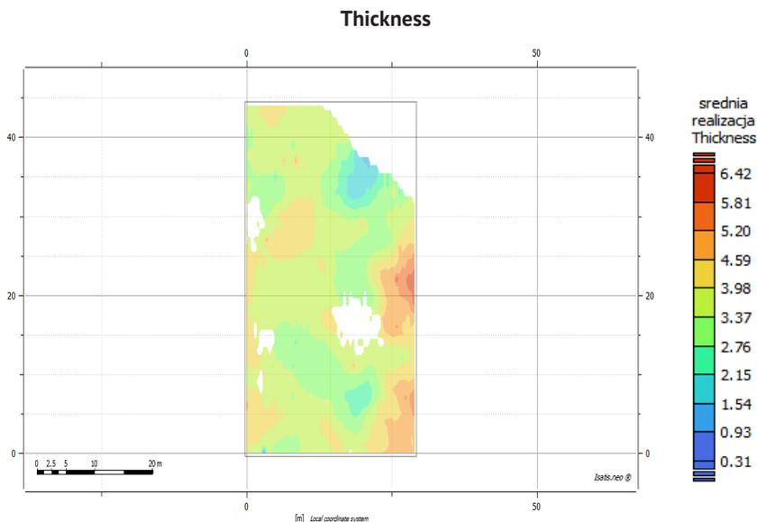
Fig. 24. Raster map of distribution of simulated values  $Z_s$  (the mean of realizations  $Z_s$ ), thickness  $th$  [m]; the R-1 block, "Rudna" mine
