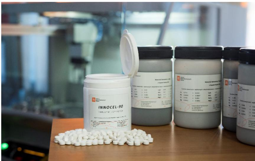
Fig. 1. Innocel-90 tablets for control of devices used in the preparation of samples for the XRF technique
