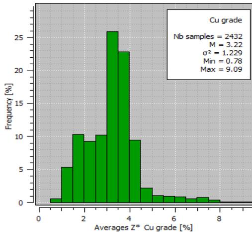
**Fig. 19.** Histogram of averages  $Z^*$  of Cu grade [%] distribution in enclosed Cu ore deposit; the block R-1, "Rudna" mine; skewness  $g_1 = 0.76$ , moderate asymmetry;  $g_2 = 5.48$ , a leptokurtic kurtosis; variation coefficient  $V = 34.46\%$
