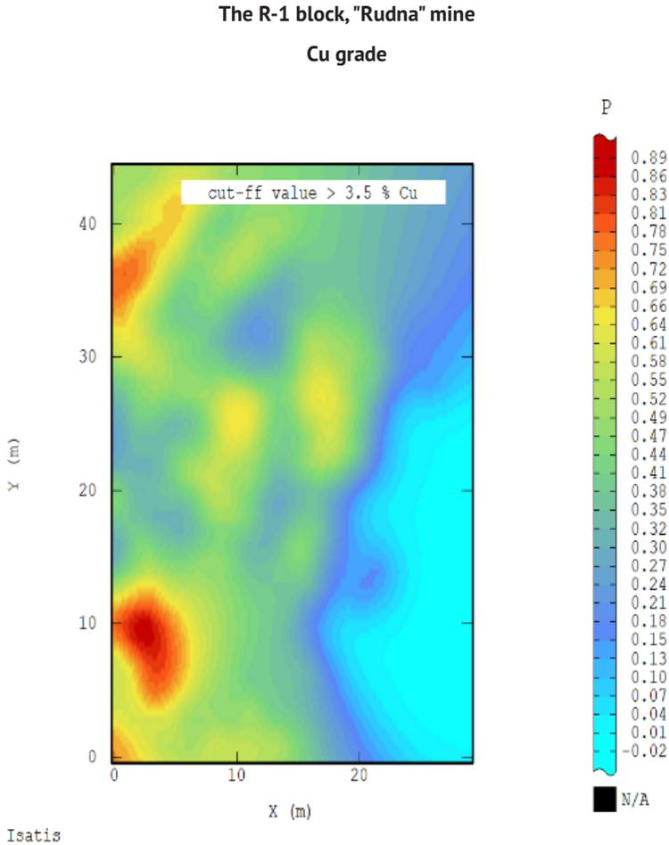
Fig. 21. Raster map of probability P distribution for the cut-off value  $> 3.5$  % Cu; copper grade [%]; the R-1 block, "Rudna" mine
