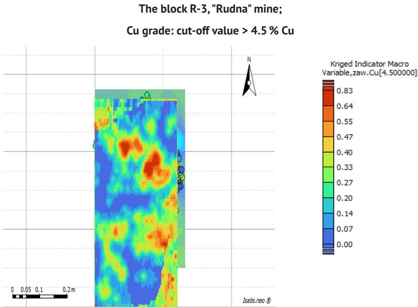
Fig. 32. Raster map of distribution of probability  $P$  of copper grade [%]: the cut-off value > 4.5 % Cu; the R-3 block, "Rudna" mine
