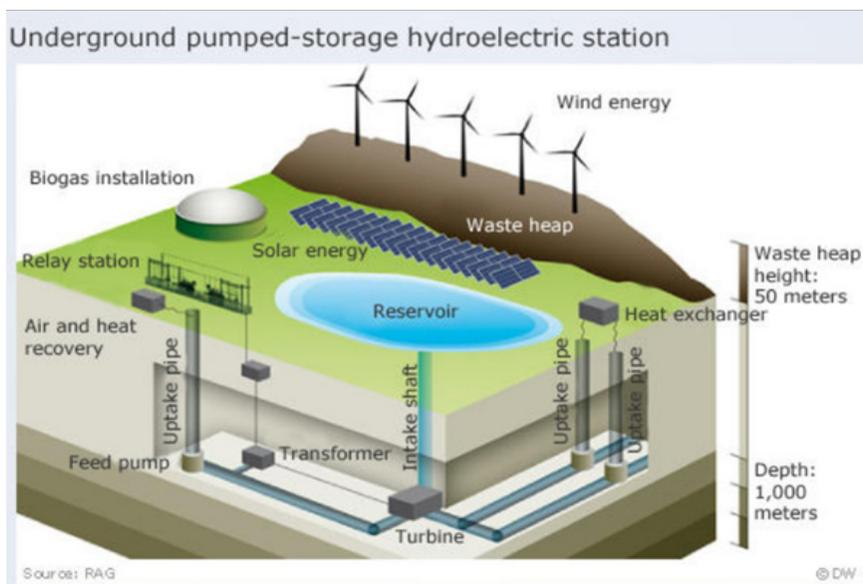
Fig. 3. Scheme of using an exploited, underground hard coal mine as electricity storage
