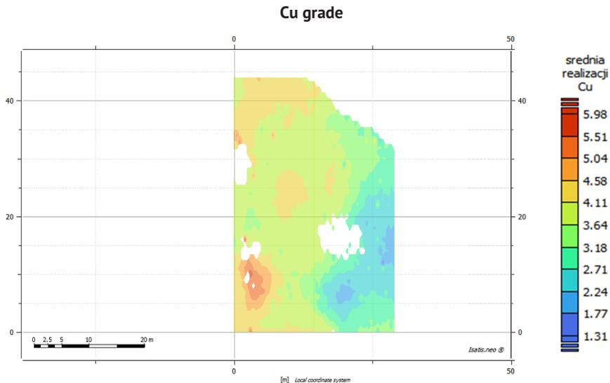
Fig. 23. Raster map of distribution of simulated values  $Z_s$  (the mean of realizations  $Z_s$ ), Cu grade [%]; the R-1 block, "Rudna" mine
