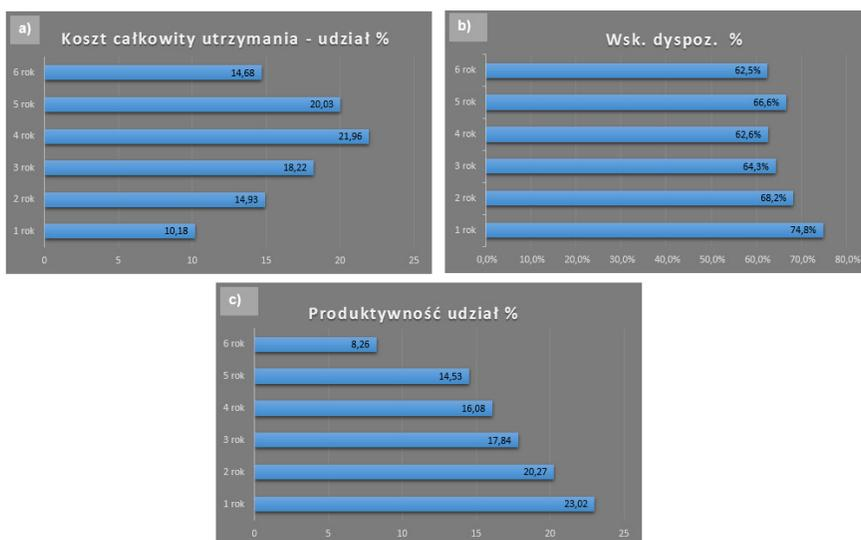
Fig. 1. Analysis of control parameters of 9 LKP-1601B machines in a 6-year operation period a) Maintenance costs, b) Availability index, c) Productivity
