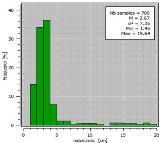
Fig. 8. Histogram of thickness [m] distribution in enclosed Cu ore deposit; the block R-1, "Rudna" mine; skewness  $g_1 = 3.85$ , strong asymmetry;  $g_2 = 18.62$ , leptokurtic kurtosis
