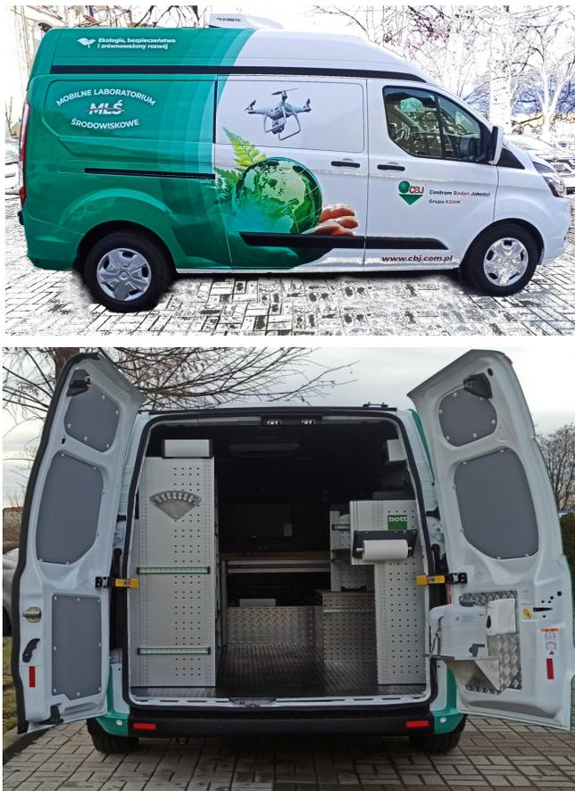
Fig. 1. An example of a car as the base and means of transport for the mobile environmental laboratory (cbj.com.pl)
