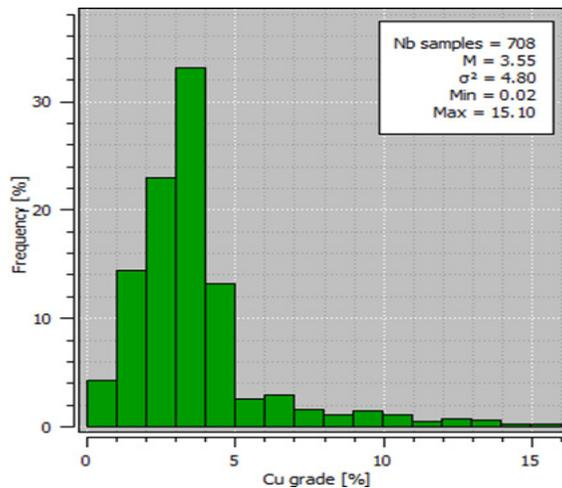
Fig. 7. Histogram of Cu grade [%] distribution in enclosed Cu ore deposit; the block R-1, "Rudna" mine; skewness  $g_1 = 2.09$ , moderate asymmetry;  $g_2 = 9.18$ , leptokurtic kurtosis
