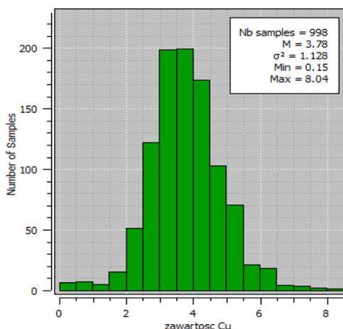
Fig. 26. Histogram of original values  $Z$  of Cu grade [%] distribution in enclosed Cu ore deposit; the block R-3, "Rudna" mine; skewness  $g_1 = 0.163$ , quasi-symmetry;  $g_2 = 4.22$ , a leptokurtic kurtosis; variation coefficient  $V = 28.07\%$
