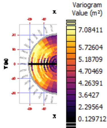
Fig. 16b. Vmap of deposit thickness [m] in copper ore deposit; R-1 block, "Rudna" mine
