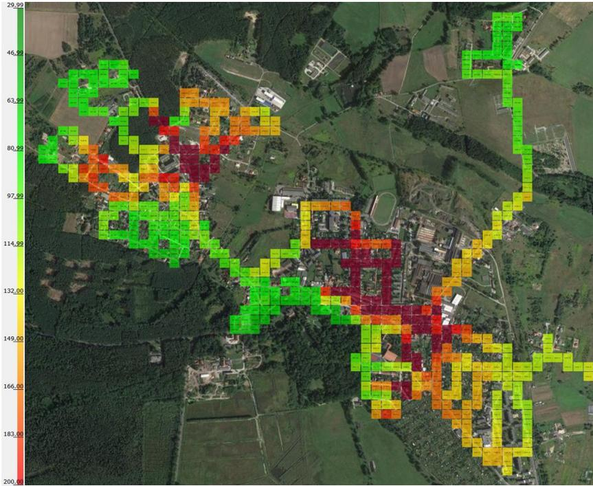
Fig. 3. Sample measurement made with an air quality analyzer. Thanks to the GPS module, after taking measurements, it is possible to accurately determine the location of the most polluted places in the entire measurement area (the darker the color, the higher the level of air pollution)
