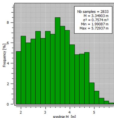
Fig. 31. Histogram of distribution of estimated averages Z\* of thickness [m]; the R-3 block, "Rudna" mine; skewness  $g_1 = 0.17$ , quasi-symmetry;  $g_2 = 2.10$ , a platokurtic kurtosis; variation coefficient  $V = 25.99\%$
