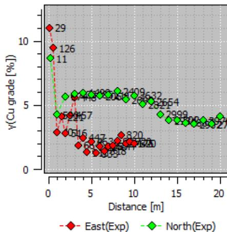
Fig.10. Two directional variograms of Cu grade [%]<sup>2</sup>; main geographical directional: N-S, W-E in enclosed Cu ore deposit; the block R-1, "Rudna" mine
