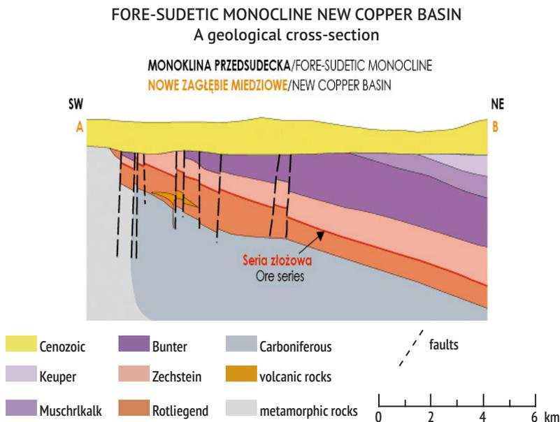
Fig. 3. A geological cross-section; Foresudetic Monocline; Copper ore series deposit is connected with the border of Whiteliengendes and Zechstein (acc. S. Oszczepalski, 1999). The deposit structure of copper-polymetallic ores is of the stratified type
