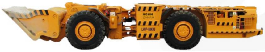
Fig. 2. LKP-0903 wheel-articulated loader by KGHM ZANAM<sup>5</sup>Table 1. Technical data of selected loaders by KGHM ZANAM<sup>6</sup>
