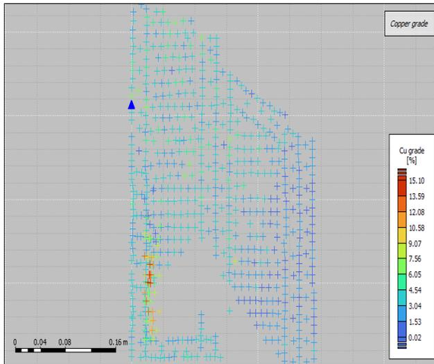
Fig. 5. Basemap with sampling points: Cu grade [%]; size N=708; distance between samples 15–20 m in the headings; The block R-1, "Rudna" mine
