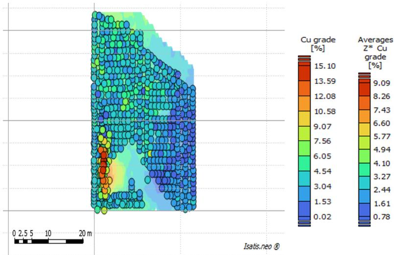
Fig. 17b. Raster map of distribution of estimated averages  $Z^*$  of Cu grade [%] with sampling points (basemap); the block R-1, "Rudna" mine; the results of ordinary (block) kriging
