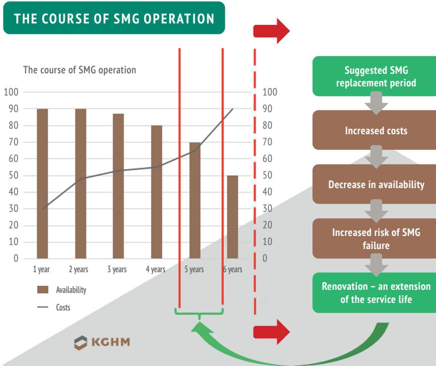
Fig. 3. The course of operation of the machine during its life in terms of the share of the unit annual cost about the total cost<sup>9</sup> [4]
