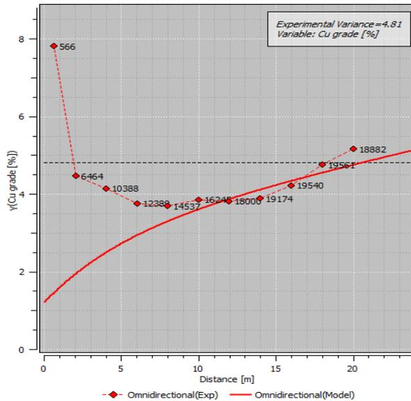
Fig. 9. Isotropic variogram of Cu grade [%]<sup>2</sup>, approximated by theoretical functions in enclosed Cu ore deposit; with parameters of the assumed model; block R-1: **exponential model**: nugget effect  $C_0 = 1.19$  [%]<sup>2</sup>, sill variance  $C' = 1.78$  [%]<sup>2</sup>; range of influence  $a = 16.22$  m; **linear model**: sill variance  $C' = 2.15$ , range of influence  $a = 23.69$  m, total sill variance  $C = 3.93$  [%]<sup>2</sup>
