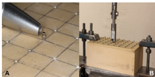
Fig. 2. A. Periotest measurement; B. The installed and separated synthetic bone block fastened to a testing machine for the pull-out test
