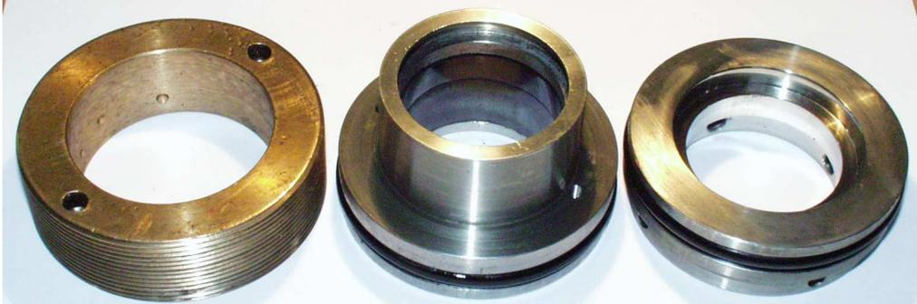
Fig. 3. Packing nut (left), stuffing-box with guide rings made of PTFE composite in closed groove (central), stuffing-box with opened groove of seal and leakage holes (left) [2]
