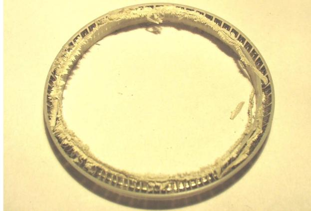
Fig. 4. Mupuseal 30412 – 0450 – 90 – S seal after 20 000 m of friction distance. Visible wear products on the seal from the guide elements made of UHMWPE [1]
