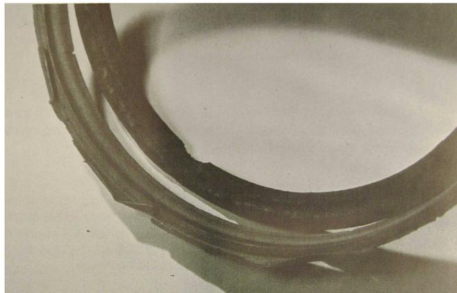
Fig. 8. Abrasive wear of the guiding ring
