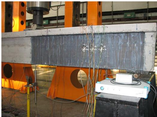
Fig. 2. Support zone of strengthened beam no. 2
