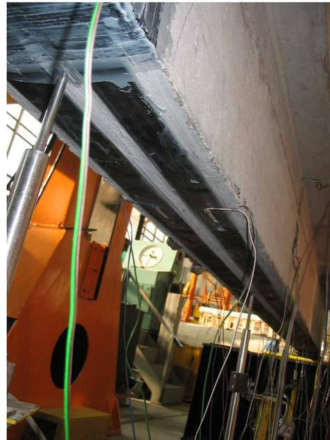
Fig. 3. Reinforcement with CFRP strips along span of beam no. 2
