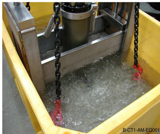
Fig. 3. System for underwater friction welding
