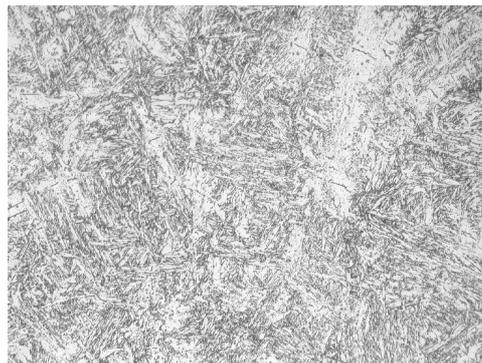
Fig. 4b The microstructure after APZ – centre of sample ( $\times 500$ )
