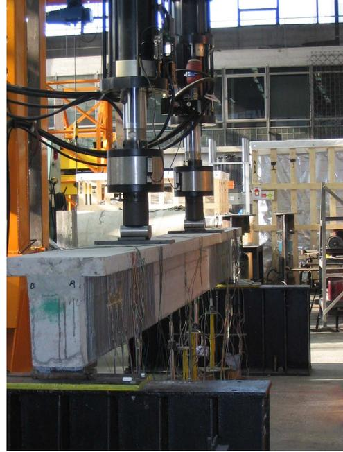
Fig. 5. Loading effected by two hydraulic servomotors
