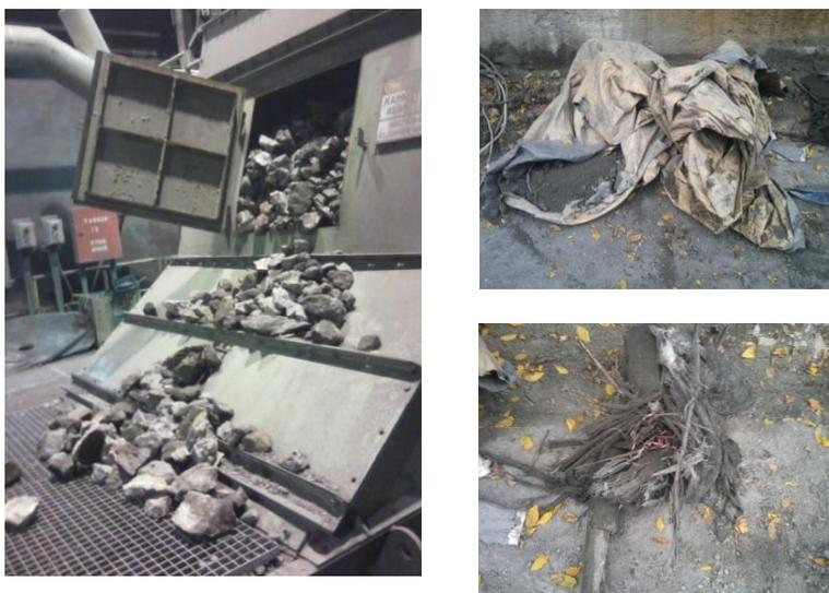
Fig. 13. Photos showing crusher and screen plugs
