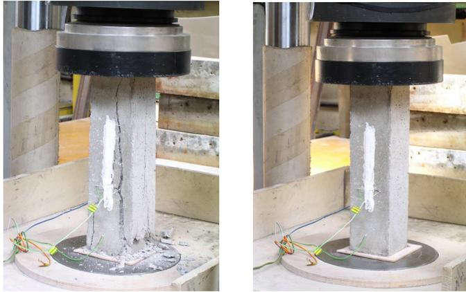
Fig. 9. Specimens of non-oiled concrete (samples) before and after the test
