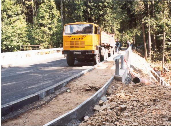
Fig. 2. Front view of bridge (without roadway layers) during test stage 1 (load scheme I)
