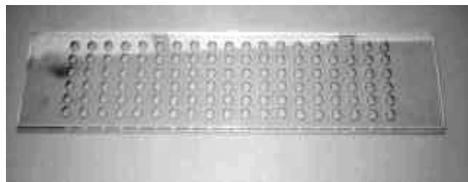
Fig. 10. Movable plate ensuring a uniform distribution of the suspension
