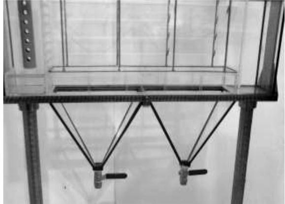
Fig.12. Hoppers for sediment collection
