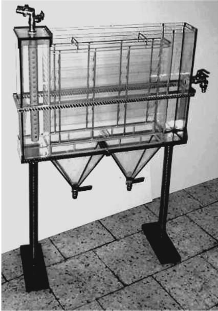
Fig. 7. Experimental set-up: sedimentation tank and a supporting structure
