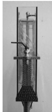
Fig. 15. Overflow-collecting pipe
