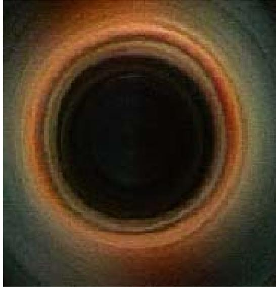
Fig. 4. Isochromatic fringe patterns at the hole of the grinding wheel rotating at the angular speed of 1150 (1/s)
