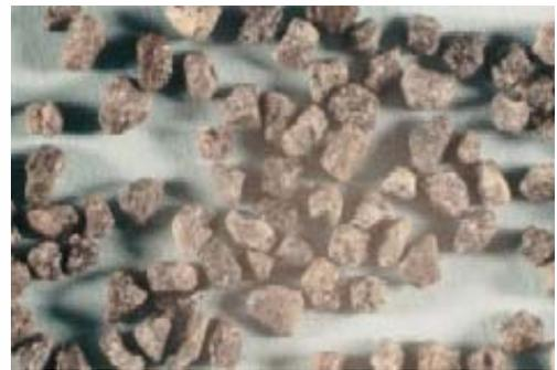
Fig. 6. Abrasant from Cubitron 321 ( $\times 10$ )
