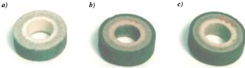
Fig. 1. The grinding wheels used in investigations: a)  $\text{Al}_2\text{O}_3$  grain, b) CBN with microcrystalline 1B grain, c) CBN with monocrystalline 3B grain
