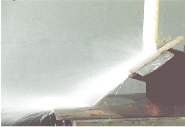
Fig. 15. Influence of a high-energy water-ice jet on a workpiece in an erosive area
