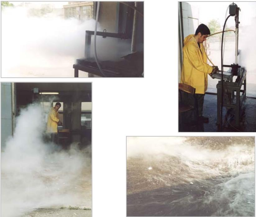
Fig. 16. Intensity of “smokiness” formed by sublimating dry-ice CO<sub>2</sub> pellets in a cleaning area while testing
