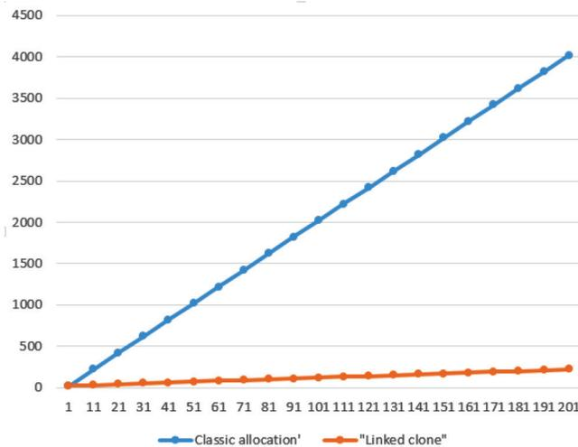
Figure 2. Estimated space required for virtual systems (in GB)
