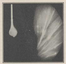
Fig. 1.—Diffraction by rocksalt. The large spot shows the position of the beam with the crystal removed.
