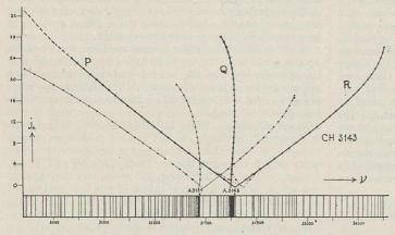
Fig. 1.—CH-band at  $\lambda 3143$ . Strong set of branches at 3143 is the 0 – 0 band. Subsidiary band at 3157 is the 1 – 1 band.
