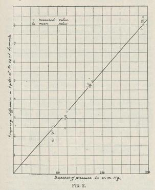
been maintained at this Laboratory since 1928. All the possible sources of frequency variation have been examined and reduced as much as possible; namely, effects due to temperature, electrical sources, output load, humidity, and surrounding conditions. The results of frequency measurement which are accurate to within one part in a million have shown that the effect of atmospheric pressure should not be neglected.
