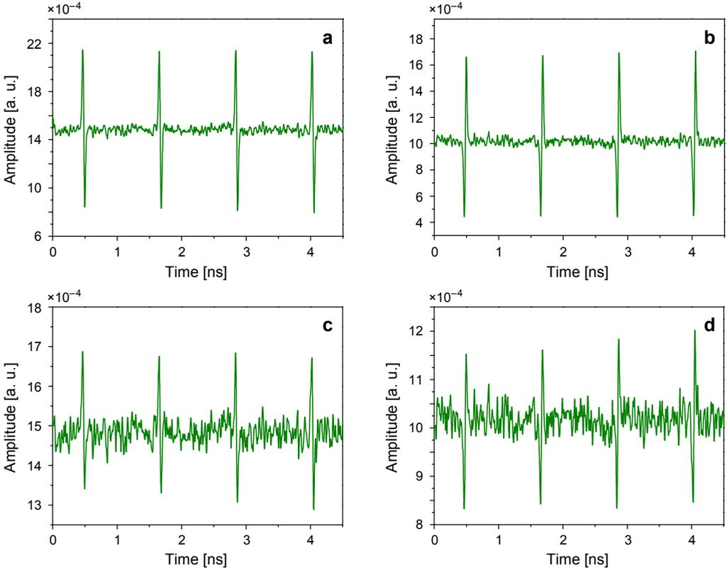
Fig. 7. Waveform diagrams of positive polarity monocycle pulse for  $\theta = 0^\circ$  (a) and negative polarity monocycle pulse for  $\theta = 0^\circ$  (b), positive polarity monocycle pulse for  $\theta = 50^\circ$  (c) and negative polarity monocycle pulse for  $\theta = 50^\circ$  (d).
