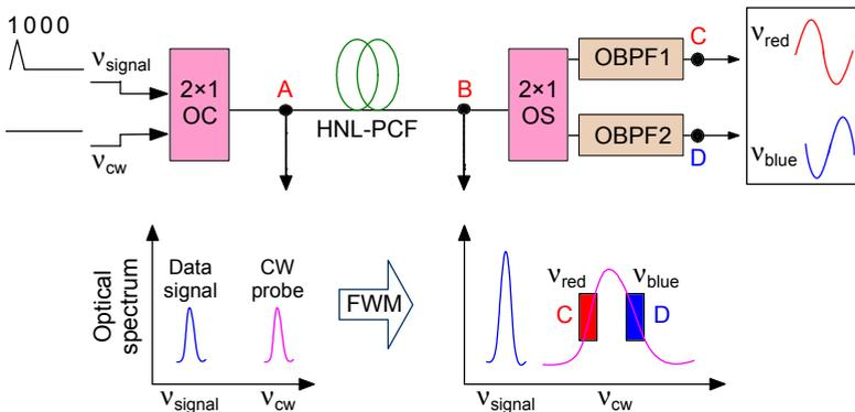
Fig. 1. Operation principle of the HNL-PCF-based polarity-reversed UWB monocycle pulse generator.
