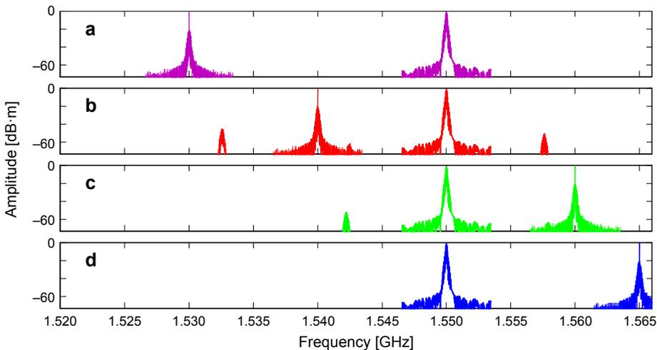
Fig. 9. Optical spectra for the dual-channel output polarity-reversed UWB monocycle pulse generator,  $\lambda_{\text{signal}} = 1550 \text{ nm}$ , and  $\lambda_{\text{cw}} = 1530 \text{ nm}$  (a),  $\lambda_{\text{cw}} = 1540 \text{ nm}$  (b),  $\lambda_{\text{cw}} = 1560 \text{ nm}$  (c),  $\lambda_{\text{cw}} = 1565 \text{ nm}$  (d).
