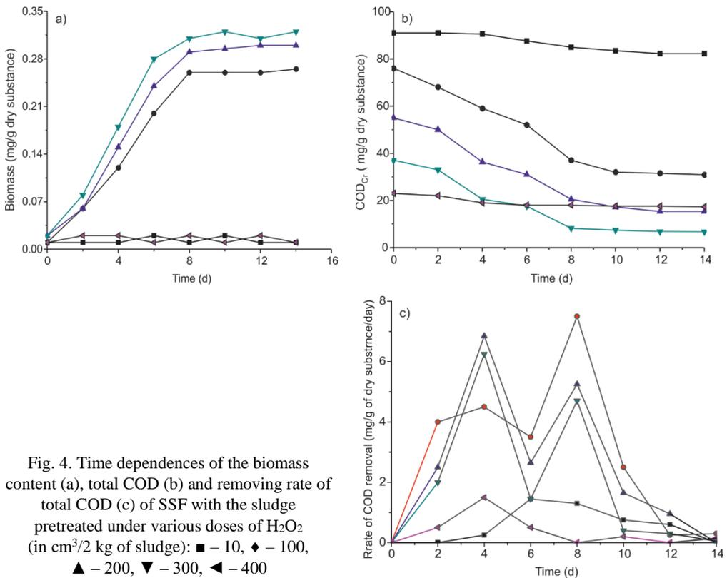
Fig. 4. Time dependences of the biomass content (a), total COD (b) and removing rate of total COD (c) of SSF with the sludge pretreated under various doses of  $H_2O_2$  (in  $cm^3/2$  kg of sludge): ■ – 10, ◆ – 100, ▲ – 200, ▼ – 300, ◀ – 400
