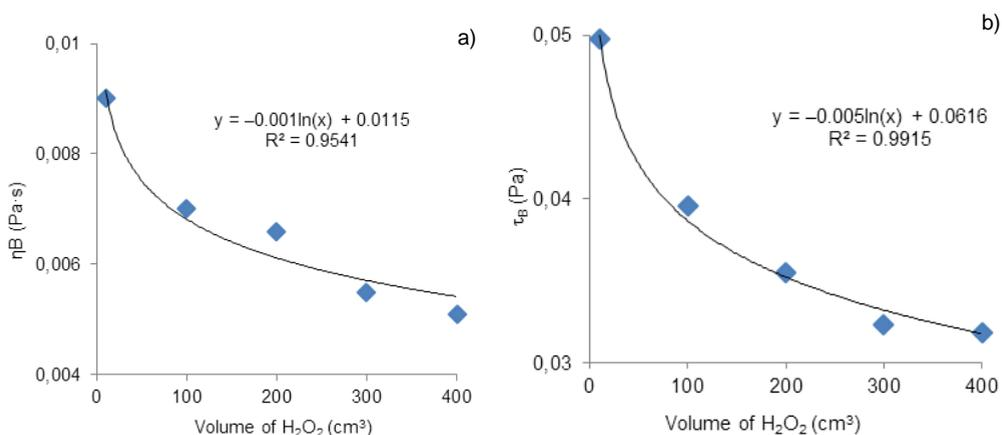
Fig. 3. Yield stress (a) and the Bingham viscosity (b) in function of the dose of  $\text{H}_2\text{O}_2$
