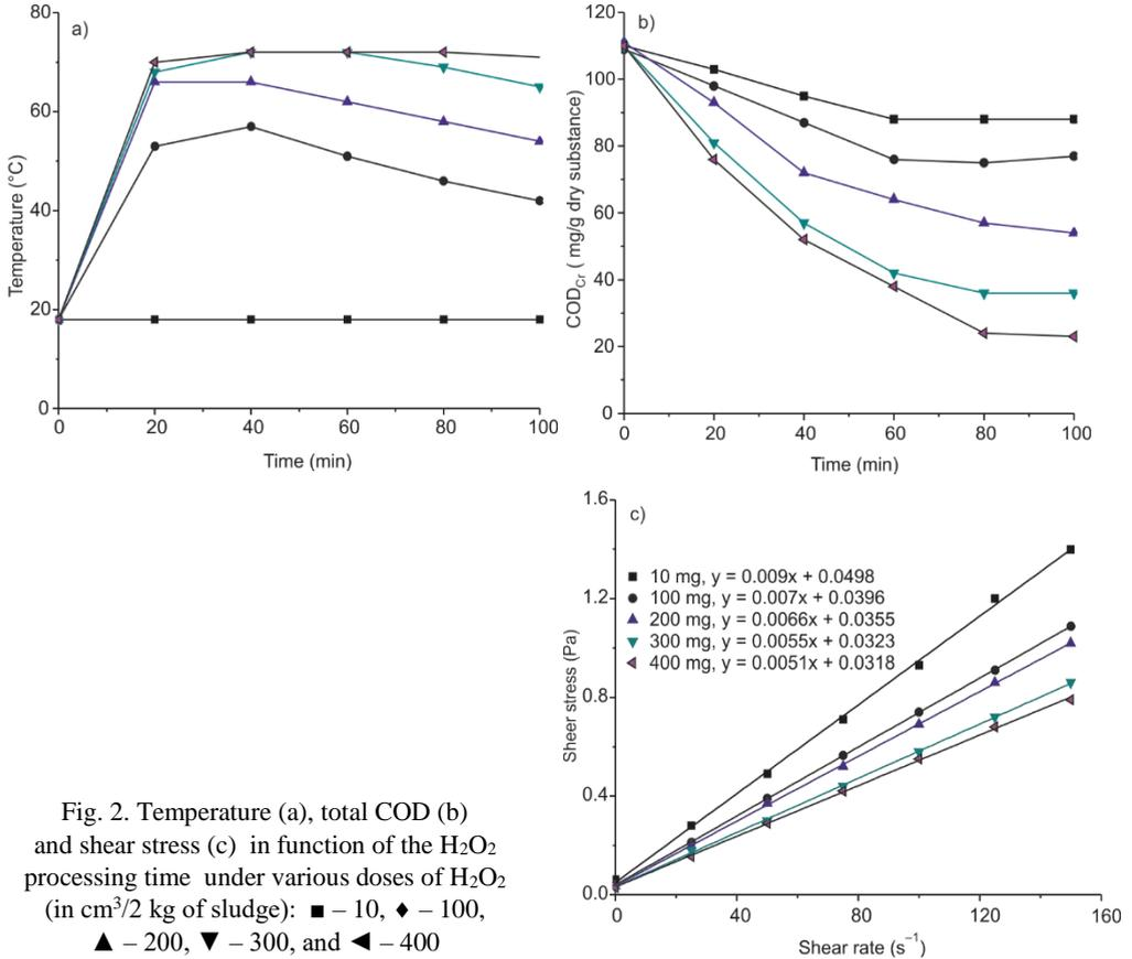
Fig. 2. Temperature (a), total COD (b) and shear stress (c) in function of the H<sub>2</sub>O<sub>2</sub> processing time under various doses of H<sub>2</sub>O<sub>2</sub> (in cm<sup>3</sup>/2 kg of sludge): ■ – 10, ◆ – 100, ▲ – 200, ▼ – 300, and ◄ – 400
