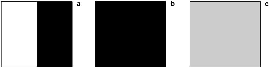
Fig. 1. Three types of shutters as solar cell shading: foil half printed black (a), foil fully printed in black (b), and foil fully printed in gray (c).
