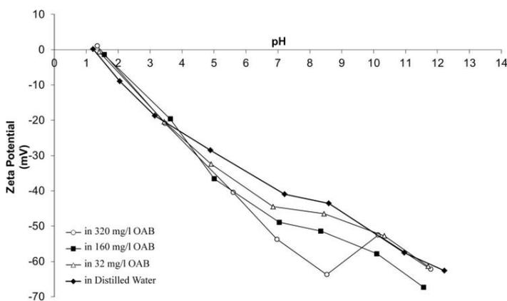
Fig. 7. Zeta potential values of orthoclase with oab collector as a function of pH
