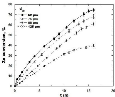
Fig. 9. Effect of mean particle size on zinc extraction.  $T = 360 \text{ K}$  ( $87 \text{ }^\circ\text{C}$ ),  $[\text{H}_2\text{SO}_4] 0.15 \text{ mol dm}^{-3}$ ,  $[\text{FeSO}_4] 0.4 \text{ mol dm}^{-3}$ , air flow rate  $0.4 \text{ dm}^3_{\text{air}} \text{ dm}^{-3}_{\text{slu}} \text{ min}^{-1}$ ,  $[\text{ZnSO}_4]_{\text{initial}} 0.025 \text{ mol.dm}^{-3}$
