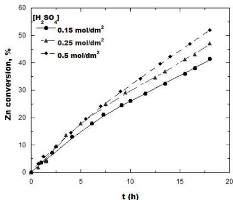
Fig. 3. Effect of sulfuric acid concentration on zinc extraction.  $T = 360 \text{ K}$  ( $87 \text{ }^\circ\text{C}$ ),  $0.025 \text{ mol dm}^{-3}$ ,  $[\text{FeSO}_4] 0.2 \text{ mol dm}^{-3}$ , air flow rate  $0.4 \text{ dm}^3_{\text{air}} \cdot \text{dm}^{-3}_{\text{slu}} \cdot \text{min}^{-1}$ , particle diameter  $88 \text{ }\mu\text{m}$
