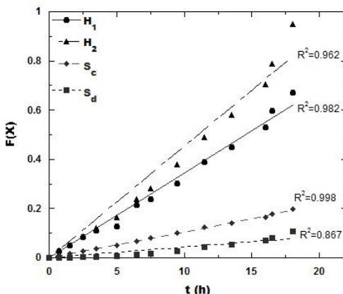
Fig. 12. Direct leaching kinetic trough pseudo-homogeneous model and shrinking core model in 360 K, [H<sub>2</sub>SO<sub>4</sub>] 0.25 mol dm<sup>-3</sup>, [FeSO<sub>4</sub>] 0.4 mol dm<sup>-3</sup>, air flow 0.4 dm<sup>3</sup><sub>air</sub> dm<sup>-3</sup><sub>slu</sub> min<sup>-1</sup>, [ZnSO<sub>4</sub>]<sub>initial</sub> 0.025 mol dm<sup>-3</sup>
