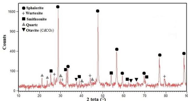
Fig. 1. XRD pattern of zinc sulfide concentrate
