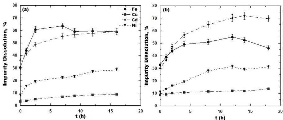
Fig. 11. Dissolution of impurities (Fe, Cu, Cd and Ni) in solution at (a) 360 K (87 °C) and (b) 368 K (95 °C).  $[\text{H}_2\text{SO}_4]$   $0.25 \text{ mol dm}^{-3}$ ,  $[\text{FeSO}_4]$   $0.4 \text{ mol dm}^{-3}$ , air flow rate  $0.4 \text{ dm}^3_{\text{air}} \text{ dm}^{-3}_{\text{slu}} \text{ min}^{-1}$ ,  $[\text{ZnSO}_4]_{\text{initial}}$   $0.025 \text{ mol dm}^{-3}$
