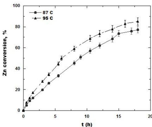
Fig. 10. Zinc extraction at 360 K (87 °C) and 368 K (95°C).
