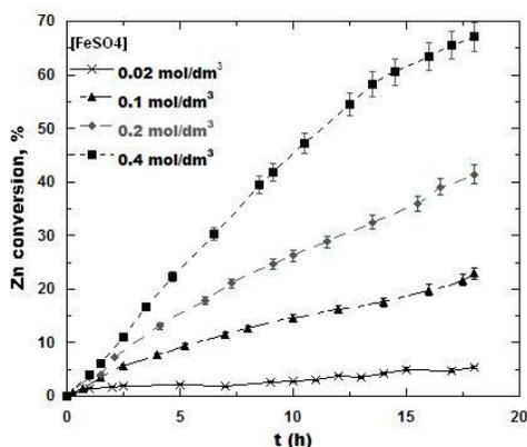
Fig. 5. Effect of ferrous sulfate initial concentration on zinc extraction.
