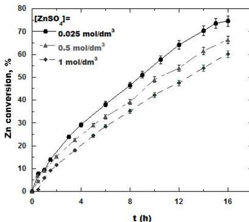
Fig. 8. Effect of zinc sulfate initial concentration on zinc extraction.  $T = 360 \text{ K}$  ( $87 \text{ }^\circ\text{C}$ ),  $[\text{H}_2\text{SO}_4] 0.15 \text{ mol dm}^{-3}$ ,  $[\text{FeSO}_4] 0.4 \text{ mol dm}^{-3}$ , air flow rate  $0.4 \text{ dm}^3_{\text{air}} \text{ dm}^{-3}_{\text{slu}} \text{ min}^{-1}$ , mean particle diameter  $52 \text{ }\mu\text{m}$
