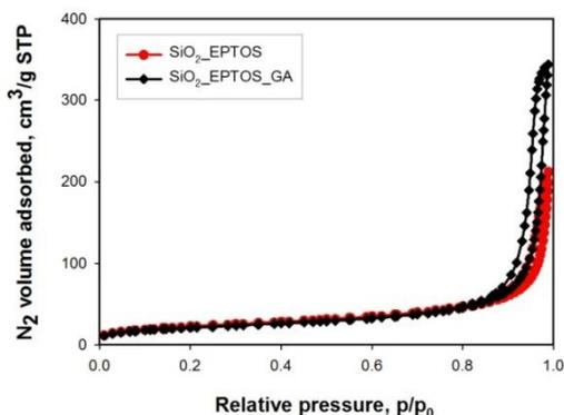
Fig. 4. Nitrogen adsorption/desorption isotherms of analyzed materials
