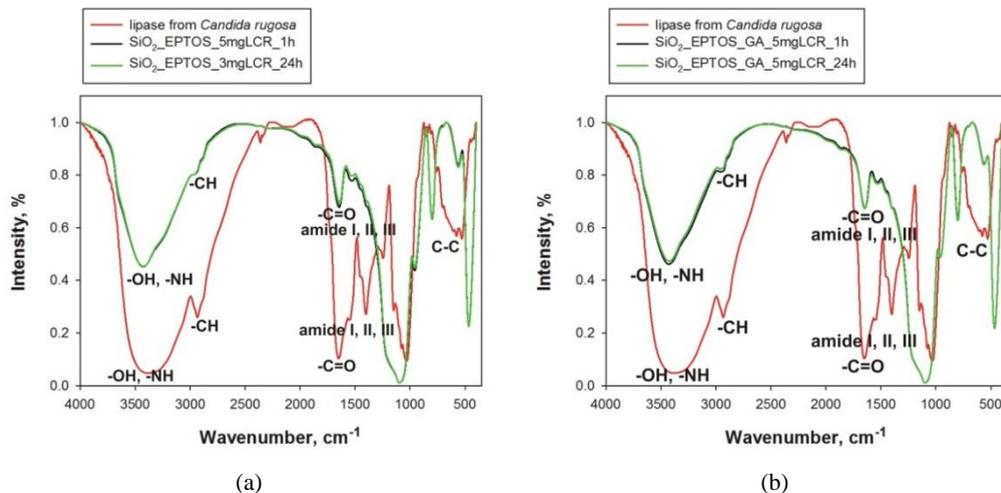
Fig. 1. FTIR spectra of lipase and lipase immobilized onto (a) SiO<sub>2</sub>\_EPTOS and (b) SiO<sub>2</sub>\_EPTOS\_GA supports
