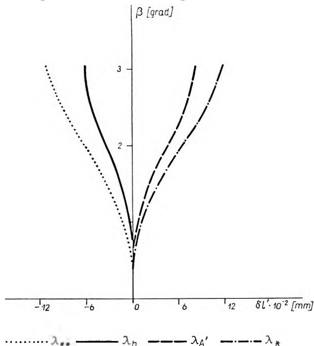
Fig. 1. Chromatic difference of the image magnitude for the superachromatic system consisting of two-lens simplets
