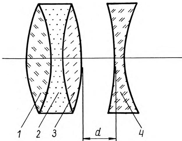
Fig. 4. Layout of the superachromat composed of two nonsuperachromatic simplets
