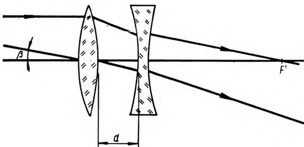
Fig. 3. Ray trace in the system composed of two thin lenses
