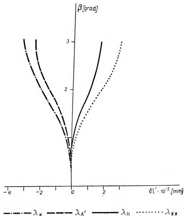
Fig. 5. Chromatic difference of the image magnitude composed of two non-superachromatic elements with an air space
