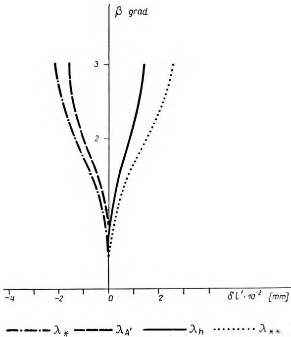
Fig. 2. Chromatic difference in the image magnitude for the three-lens simplets
