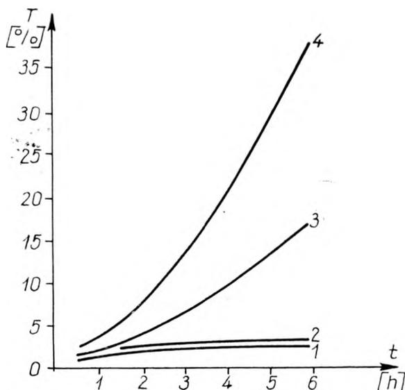
Fig. 3. Behaviour of the dye TE-25 in nitrobenzene in function of time: 1 and 2 — measurements in darkness, 3 and 4 — measurements in illumination  $T_1 = T_3 < T_2 = T_4$
