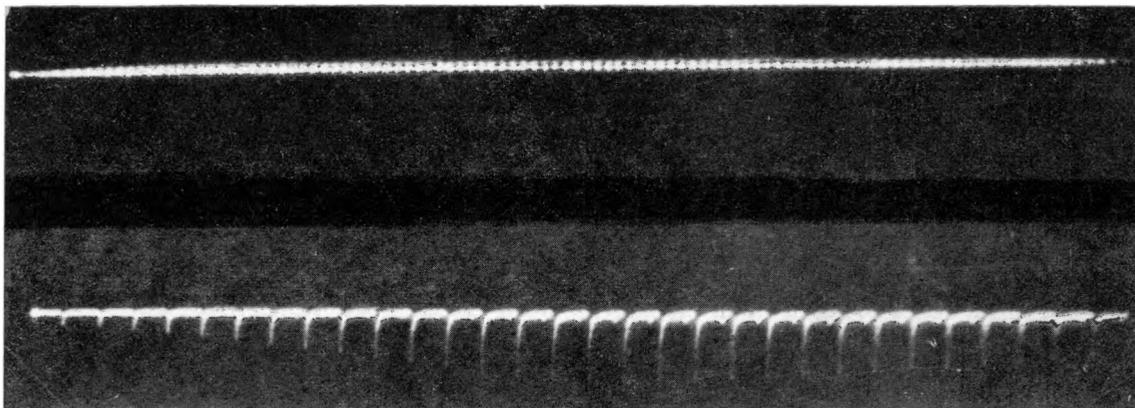
Fig. 8. Pulse train in arrangement with self-synchronization of modes. The upper path shows for comparison the 10 ns time markers
