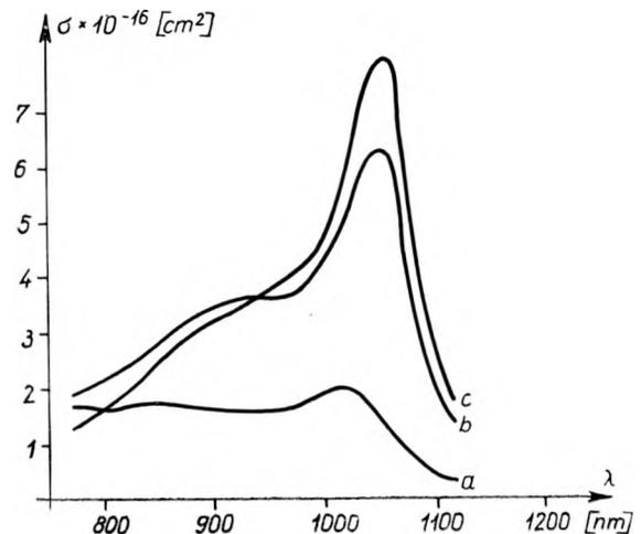
Fig. 2. Unitary absorption of the dye TE-26 solution in various solvents: *a* — in methanol, *b* — in nitrobenzene, *c* — in quinoline
