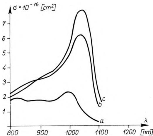
Fig. 1. Unitary absorption of the dye TE-25 solution in various solvents: *a* — in methanol, *b* — in nitrobenzene, *c* — in quinoline
