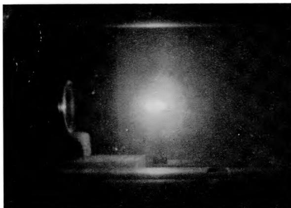
Fig. 7. The air ionization effect by concentrated laser radiation. Lens of focal length  $f = 150$  mm
