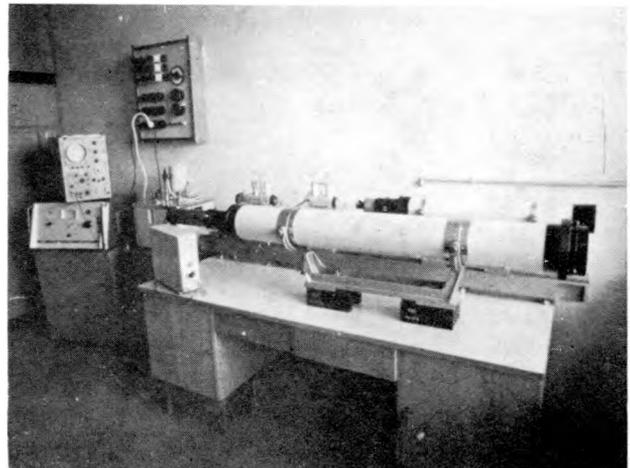
Fig. 4. Laboratory measuring setup of Raman Lidar
