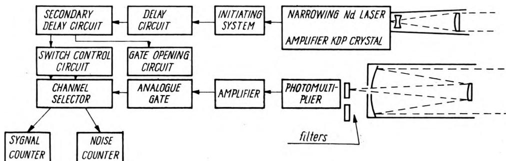
Fig. 3. Principle of Raman Lidar operation
