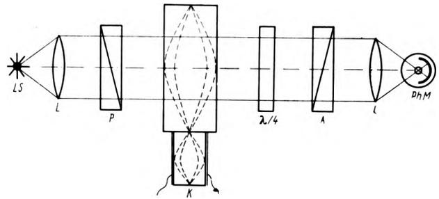
Fig. 1. Elastooptic light modulator
