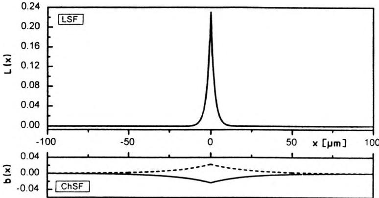
Fig. 2. Comparison of the LSF and ChSF. The ChSF for development-inhibiting compounds – solid lines, the ChSF for development-accelerating compounds – dashed lines.
