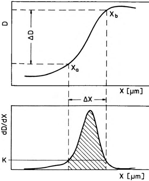
Fig. 8. Image of a knife-edge exposure used to measure acutance.  $\Delta D$  is the density difference over the distance  $\Delta X$ .
