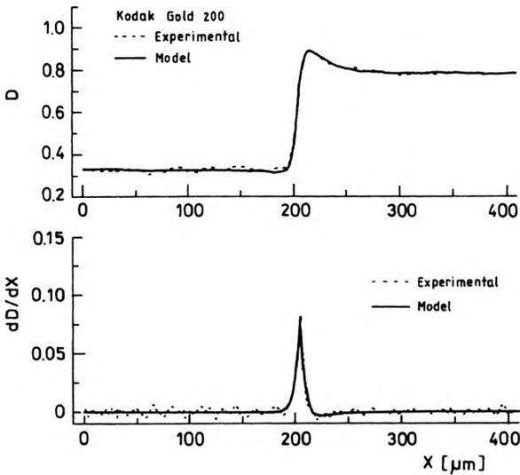
Fig. 6. Comparison of (a) experimental edge densities and their differentials (dashed lines), and the corresponding (b) model edge densities and their differentials (solid lines). Experimental made on colour negative Kodak Gold 200. The parameters of modelling are as follows:  $K = 20$ ,  $K_c = 90$ ,  $R = 5.28\%$  ChSF in ESF.
