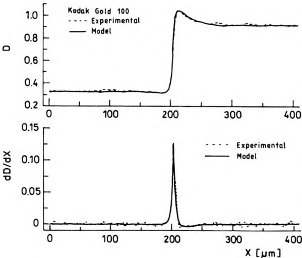
Fig. 5. Comparison of (a) experimental edge densities and their differential (dashed lines) and the corresponding (b) model edge densities, and their differentials (solid lines). Experiment made on colour negative Kodak Gold 100. The parameters of modelling are as follows:  $K = 15$ ,  $K_c = 90$ ,  $R = 6.24\%$  ChSF in ESF.
