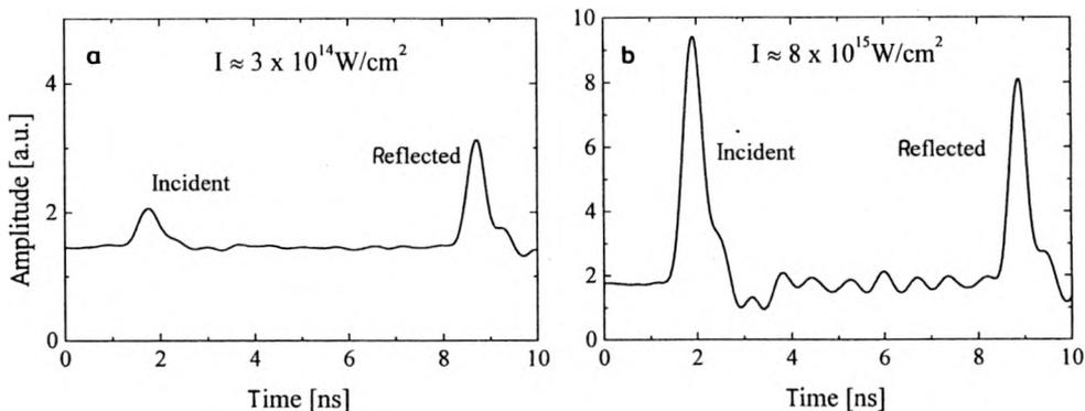
Fig. 2. Oscillograms of incident and reflected pulses at two different intensities of light on the target.
