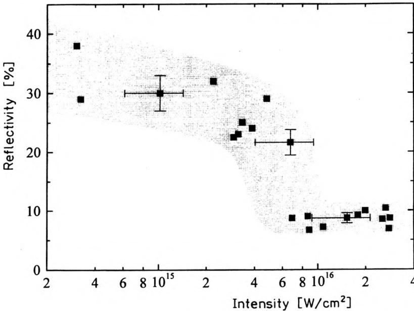
Fig. 3. Specular reflectivity as a function of light intensity on the target.
