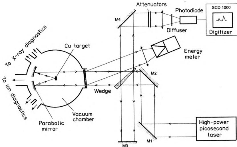
Fig. 1. Experimental arrangement for measurements of reflectivity of a high-intensity picosecond light pulse from a metal target.
