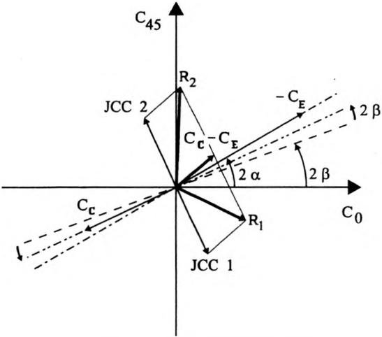
Fig. 7. Same as in Fig 4, but as a result of the new axis setting  $\beta'$  of the trial cylinder. The trial cylinder has been rotated from the position in Fig. 4 towards the minus axis of the JCC position that provided better vision.
