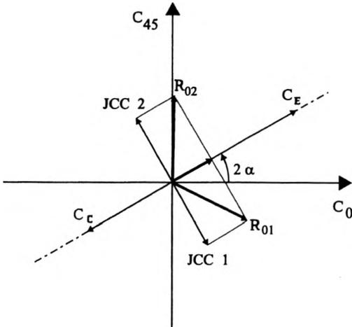
Fig. 6. Reference situation for the proper position of the trial cylinder axis. The resultant  $R_{01}$  and  $R_{02}$  of the two flip positions of the JCC produce the same blur and the patient will show no preference for one position over the other.
