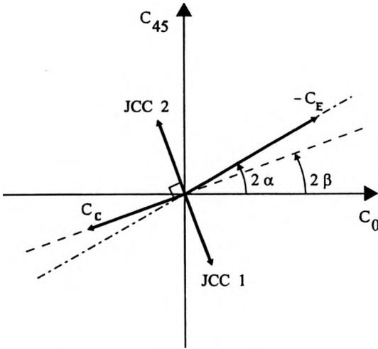
Fig. 4. Cylinder axis refinement with the Jackson cross cylinder represented in the JCCs plane of the dioptric power space.  $C_R$  is the astigmatic refractive error.  $C_C$  is the erroneous correcting cylinder. JCC1 and JCC2 represent the Jackson cross cylinder with their axes forming  $\pm 45^\circ$  with  $C_C$ .
