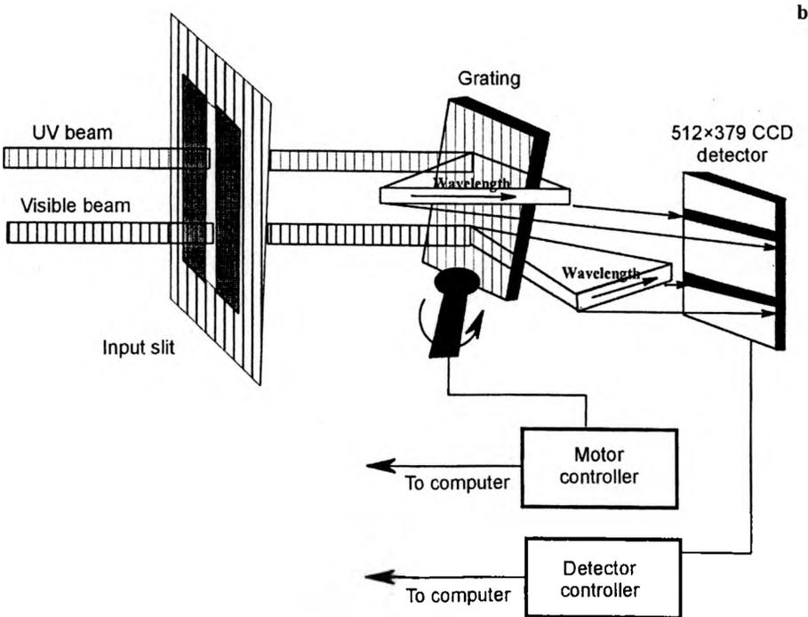
Fig. 1. Block diagram for the experimental setup (a). Optical paths of the UV and visible beams inside the spectrograph (b).
