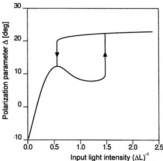
Fig. 4. Theoretical dependence of phase difference  $\Delta$  (in degrees) between two linear components of polarization of the output light as a function of the input light intensity, for the case of electric vector  $\mathbf{E}$  of input light perpendicular to the director  $\mathbf{n}$  of the liquid crystal. Light intensity is in arbitrary units  $(\Gamma L)^{-1}$ .
