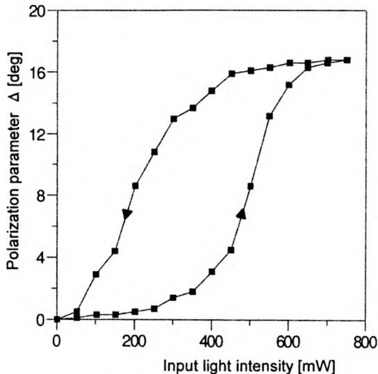
Fig. 3. Phase difference  $\Delta$  (in degrees) between two linear components of polarization of the output light as a function of the input light intensity, measured for the electric vector  $\mathbf{E}$  of input light perpendicular to the director  $\mathbf{n}$  of the liquid crystal.
