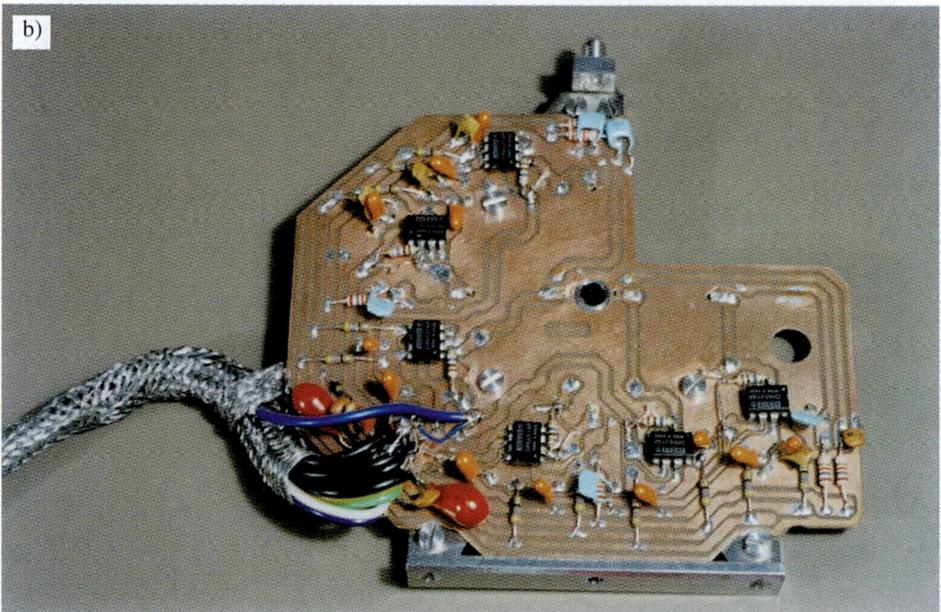
Fig. 2. The detector system view from: a) the p-i-n diodes side; b) the preamplifiers side
