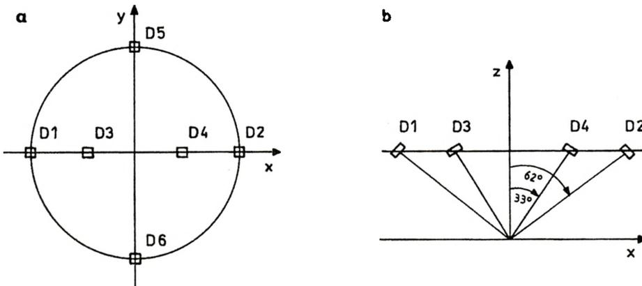
Fig. 1. Arrangement of detectors in relation to the coordinate system x-y-z: a – top view, b – detection angles quantity.
