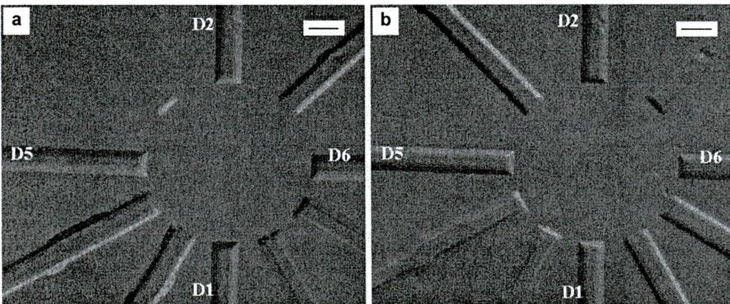
Fig. 6. Surface digital images with radially located grooves in case where: a – TOPO mode is produced according to the algorithm  $(D2-D1)+(D6-D5)$ , b – TOPO mode is produced according to the algorithm  $(D1-D2)+(D6-D5)$  (bar = 50  $\mu\text{m}$ ).
