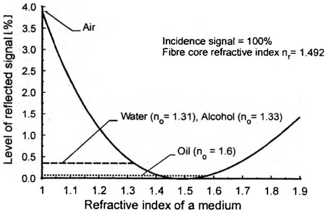
Fig. 3. Reflected signal from a submersed head.
