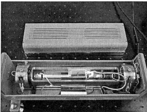
Fig. 4. Laser head of the laser frequency standard.
