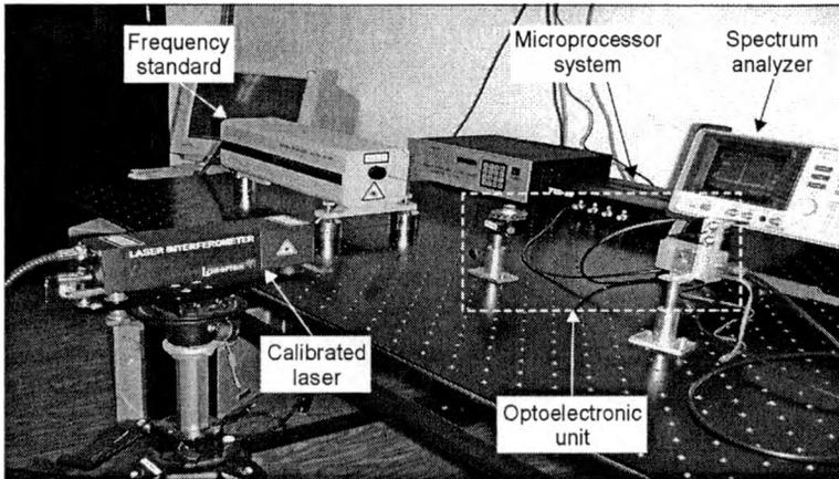
Fig. 1. Laser calibration system.
