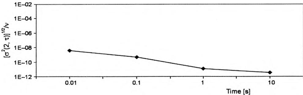
Fig. 6. Results of the measurements of the laser frequency stability of the standard.
