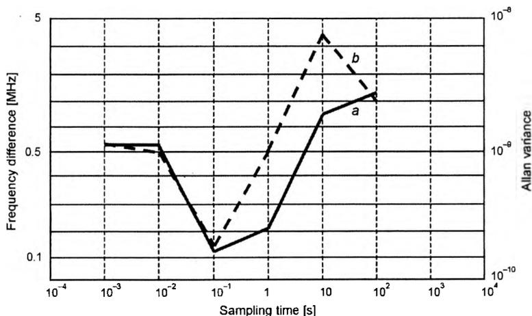
Fig. 8. He-He Zeeman laser frequency stability: digital method (a) and analog method (b).
