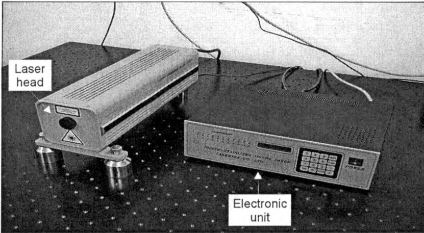
Fig. 3. Iodine stabilized He-Ne laser at  $\lambda = 633$  nm.
