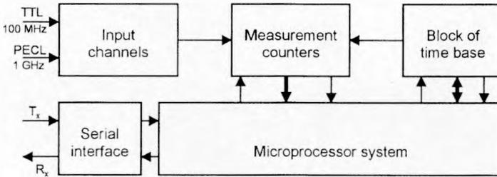
Fig. 2. Block diagram of the microprocessor system.
