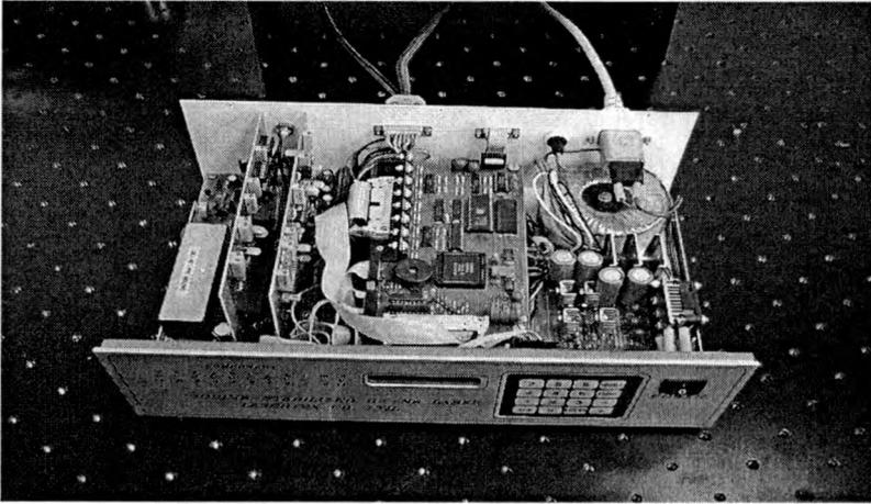
Fig. 5. Electronic unit of the laser frequency standard.
