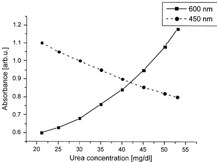
Fig. 3. Calibration curves. The absorbance vs. urea concentration recorder for 450 and 600 nm.
