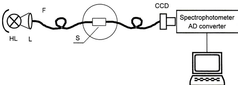
Fig. 1. Experimental set-up. HIL – halogen light source, L – coupling lens, F – optical fiber, S – container with urea solution and an optode, CCD – detector connected with the computer.
