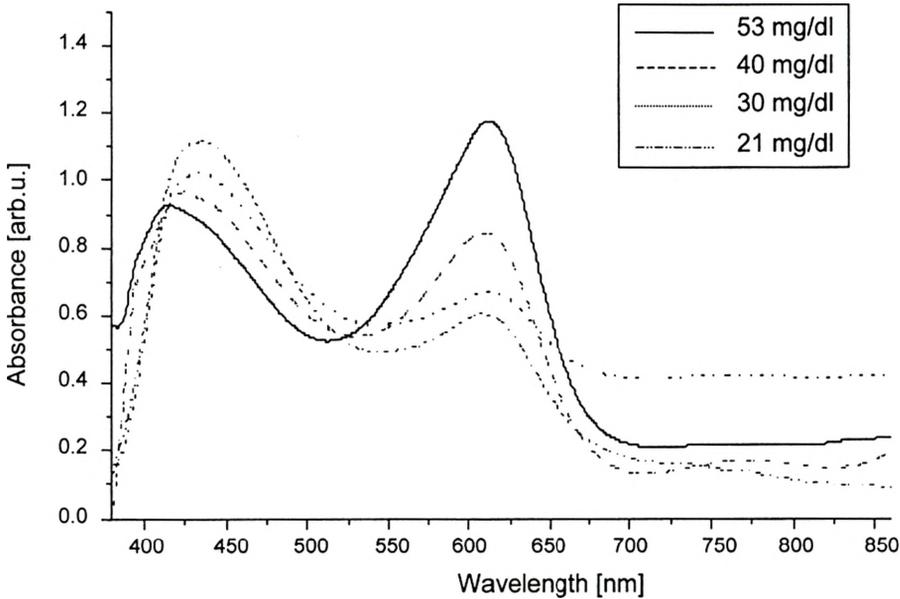
Fig. 2. Absorbance of an optode (urease and bromothymol blue as an indicator entrapped in a sol-gel matrix) in the presence of urea in the environment.
