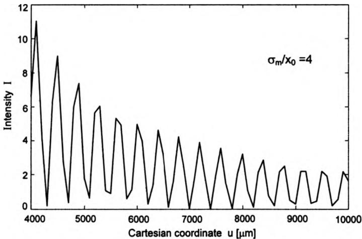
Fig. 8. Magnified portion of the intensity distribution  $I(u)$  in the range from  $u = 4000 \mu\text{m}$  up to  $10000 \mu\text{m}$  ( $\sigma_m = 10 \mu\text{m}$  and  $x_0 = 2.5 \mu\text{m}$ ).
