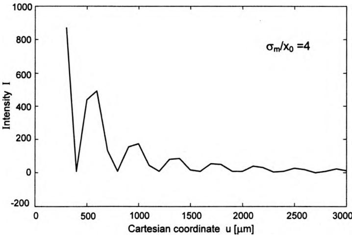
Fig. 7. Magnified portion of the intensity distribution  $I(u)$  in the range from  $u = 300 \mu\text{m}$  up to  $3000 \mu\text{m}$  ( $\sigma_m = 10 \mu\text{m}$ ,  $x_0 = 2.5 \mu\text{m}$ ).
