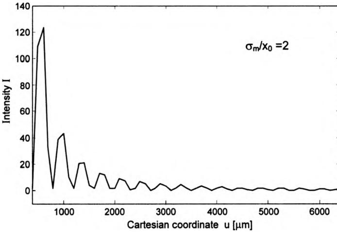
Fig. 4. Intensity distribution of the diffraction pattern vs. Cartesian coordinate  $u$  for an inverted parabolic shape of height  $\sigma_m = 5 \mu\text{m}$  and half width  $x_0 = 2.5 \mu\text{m}$  in the range from  $300 \mu\text{m}$  up to  $6300 \mu\text{m}$ .
