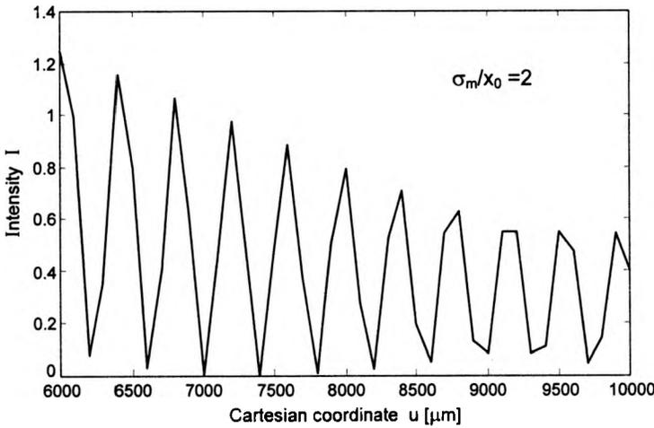
Fig. 5. Intensity distribution of the diffraction pattern vs. Cartesian coordinate  $u$  for an inverted parabolic shape of height  $\sigma_m = 5 \mu\text{m}$  and half width  $x_0 = 2.5 \mu\text{m}$  in the range from  $6000 \mu\text{m}$  up to  $10000 \mu\text{m}$ .
