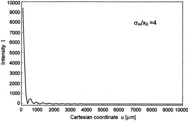
Fig. 6. Intensity distribution of the diffraction pattern vs. Cartesian coordinate  $u$  for an inverted parabolic shape of height  $\sigma_m = 10 \mu\text{m}$  and half width  $x_0 = 2.5 \mu\text{m}$ .
