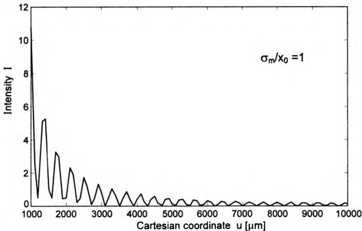
Fig. 3. Magnified portion of the intensity distribution  $I(u)$  in the range from  $u = 1000 \mu\text{m}$  up to  $10000 \mu\text{m}$  ( $\sigma_m = 2.5 \mu\text{m}$  and  $x_0 = 2.5 \mu\text{m}$ ).
