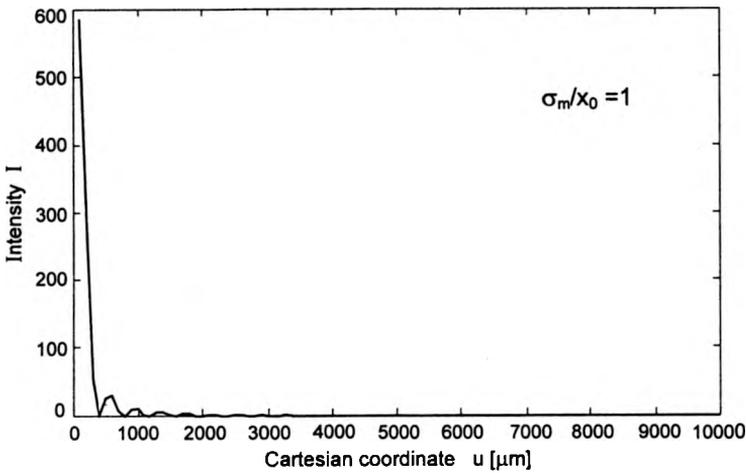
Fig. 2. Intensity distribution of the diffraction pattern vs. Cartesian coordinate  $u$  for an inverted parabolic shape of height  $\sigma_m = 2.5 \mu\text{m}$  and half width  $x_0 = 2.5 \mu\text{m}$ .
