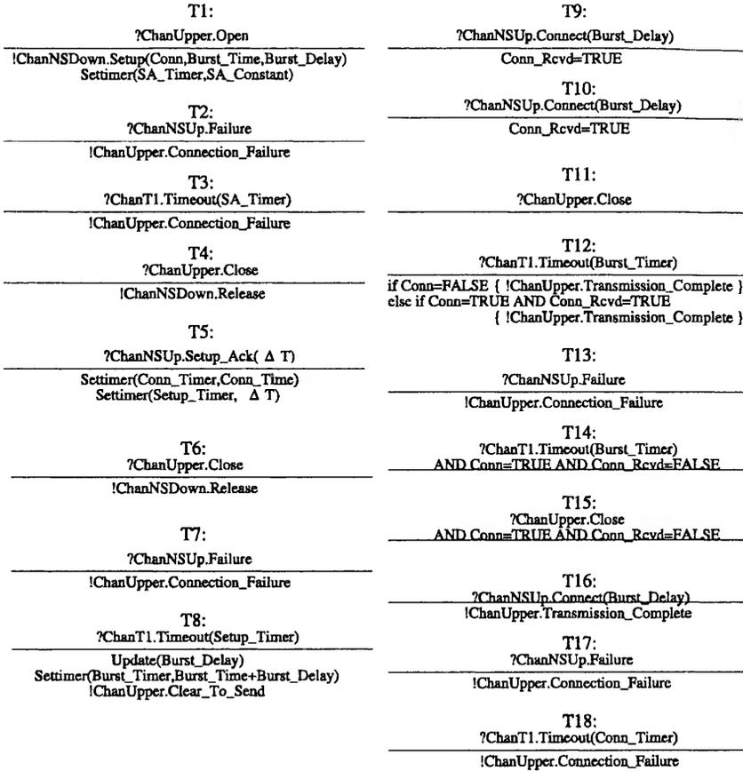
Fig. 4. State transitions for source client.
