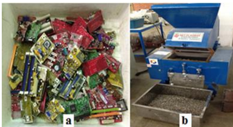
Fig. 2. Manually sorted PCB's (a) and shredder (b)
